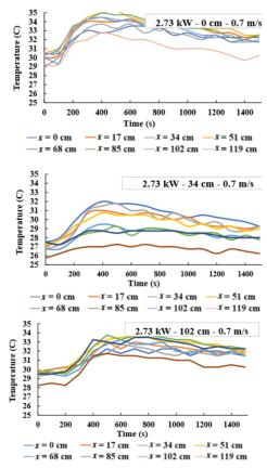
Fig. 6. Temperature profile of 2.73 kW fire at 0.7 m/s for different fire source locations.
