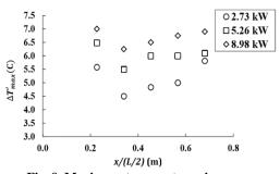
Fig. 9. Maximum temperature rise versus various dimensionless longitudinal fire locations.
