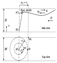
Fig. 3. Fire plume schematic view.
