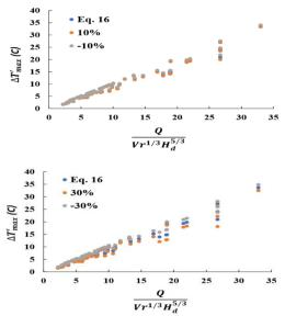
Fig. 13. Comparison between calculated maximum thermal smoke temperature rises with  $\pm 10$  changes in  $\frac{x}{L/2}$  and  $\pm 30$  changes in  $\frac{x}{L/2}$ .
