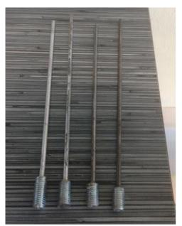
Fig. 6. Aluminium and carbon steel cylinders with AR = 50 and 54.
