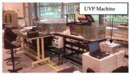
Fig. 2. Recirculating water channel.
