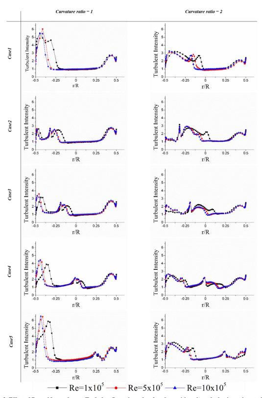
Fig. 3. Effect of Reynolds number on Turbulent Intensity at bend outlet position along the horizontal centerline from inner to outer curvature wall side (r/R value -0.5 represents the inner side and 0.5 as outer side).
