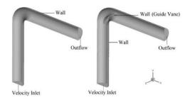
Fig. 1. A representative diagram of the bend geometry (a) Without Guide Vane and (b) With guide vane
