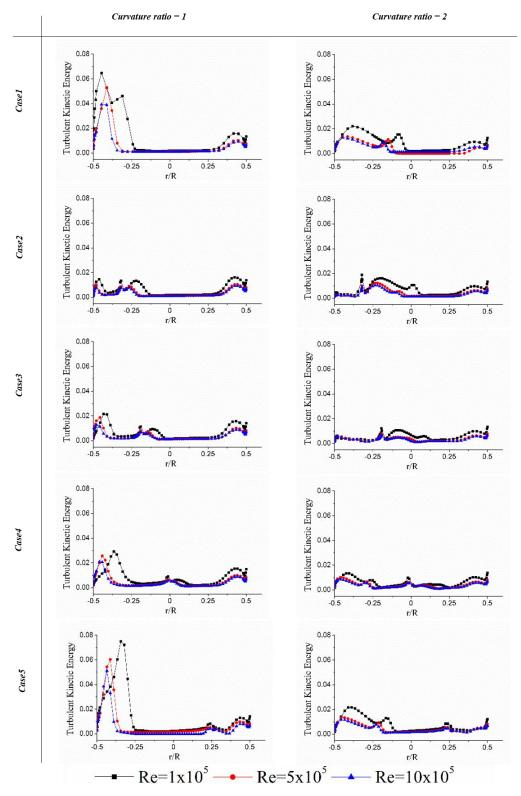
Fig. 4. Effect of Reynolds number on Turbulent Kinetic Energy at bend outlet position along the horizontal centerline from inner to outer curvature wall side (r/R value -0.5 represents the inner side and 0.5 as outer side).
