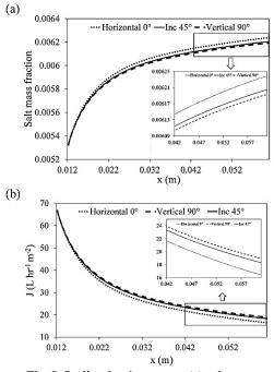
Fig. 8. Inclination impact on (a) salt mass
