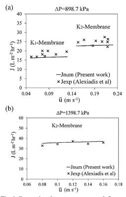
Fig. 4. Comparison between present work  $J_{num}$ and experimental study  $J_{exp}$  for different crossflow velocities at (a) low transmembrane pressures including  $K_1$  and  $K_2$  – membranes and (b) high transmembrane pressures for  $K_2$  – membrane.
