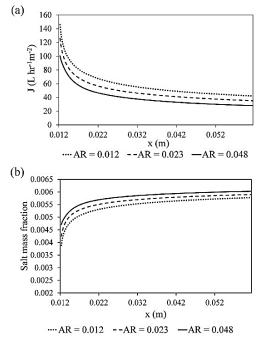
Fig. 7. Aspect Ratio effect on (a) permeate flux and (b) salt mass fraction distribution along the membrane.
