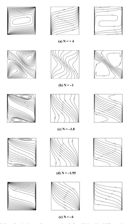
$\begin{array}{l} \textbf{Fig. 2. Streamlines, isotherms and iso-concentrations for } R_T = 400, Le = 10 \text{ and different values of } N\text{: a)} \\ N = +4 \left(\Psi_{min} = 0, \Psi_{max} = 16.48\right), b) \ N = -1 \left(\Psi_{min} = -1.66, \Psi_{max} = 4.30\right), c) \ N = -1.8 \left(\Psi_{min} = -3.34, \Psi_{max} = 0.47\right), d) \ N = -1.95 \left(\Psi_{min} = -3.60, \Psi_{max} = 0.067\right), and e) \ N = -4 \left(\Psi_{min} = -6.85, \Psi_{max} = 0\right). \end{array}$
