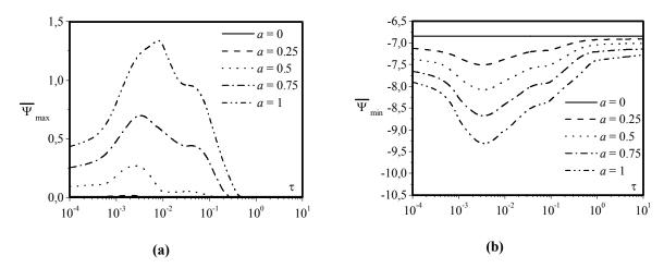
Fig. 8. Variation of the maximum (a) and minimum (b) stream functions with the period  $\tau$  for Le = 10, N = -4,  $R_T = 400$  and different values of the amplitude a.
