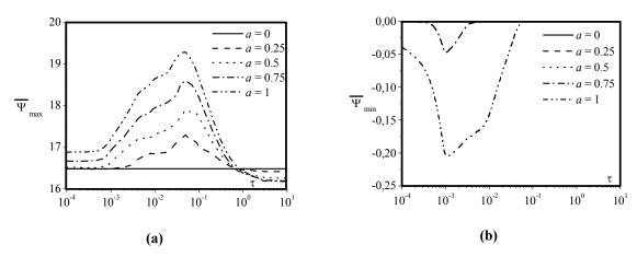
Fig. 6. Variation of the maximum (a) and minimum (b) stream functions with the period  $\tau$  for Le = 10, N = +4,  $R_T = 400$  and different values of the amplitude a.
