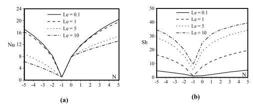
Fig. 3. Overall Nusselt number Nu (a) and Sherwood number Sh (b) as functions of buoyancy ratio N for the case  $R_T = 400$  with the Lewis number as parameter.
