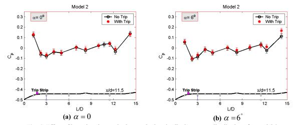
Fig. 4. Effect of boundary layer tripping on the longitudinal pressure distributions for model 2.
