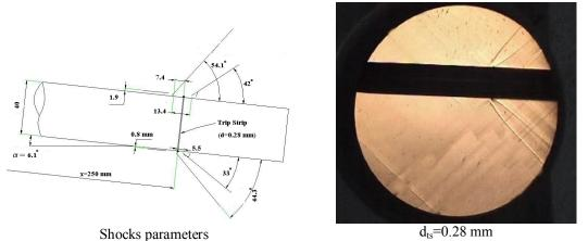
Fig. 7. Illustration of angles, distances and forms of the shocks relative to themselves and body, for the model 1 with 0.28 mm in diameter trip strip installed at x/d=6.25 and at  $\alpha = 6^{\circ}$ .
