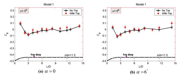
Fig. 9. Effect of boundary layer tripping on longitudinal pressure distributions for model 1.
