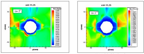
(a) Clean Model (b) Model with trip strip Fig. 8. Effect of boundary layer tripping on Mach contours at x/d=11.25 and  $\alpha = 2^{\circ}$ , for Model 2.
