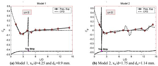
Fig. 8. Comparison of the experimental and the numerical longitudinal pressure distributions at  $\alpha = 0$ .
