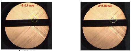
$d_{ts}=0.9 \text{ mm}$   $d_{ts}=0.28 \text{ mm}$ Fig. 6. Flow around cylindrical part of the Model 1 with trip strip installed at x/6=6.25 and  $\alpha = 0$ .
