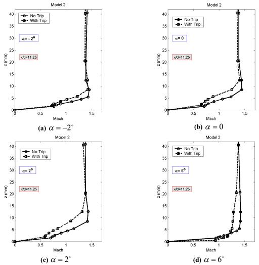
Fig. 7. Comparison of the boundary layer profiles for with/without trip strip on model 2 at x/d=11.25.
