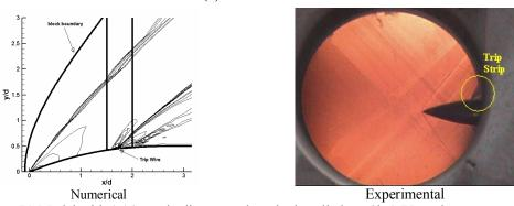
(b) Model with 1.14 mm in diameter trip strip, installed at x/d=1.75 on the nose Fig. 5. Experimental (Schlieren photograph) and numerical (pressure contours) flow field over the nose of the model at  $\alpha = 0$ .
