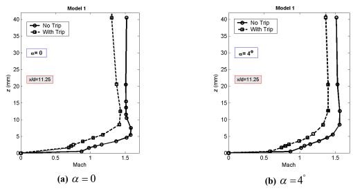
Fig. 6. Comparison of the boundary layer profiles for with/without trip strip on model 1 at x/d=11.25.
