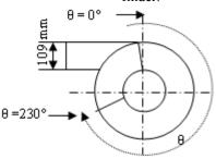
**Fig. 3.** Angular measuring positions:  $-10^{\circ} < \theta < 230^{\circ}$  by steps of 20°.
