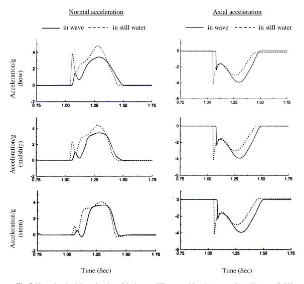
Fig. 7. Normal and axial acceleration of the boat at different positions in wave and in still water ( $\theta$ =30°, H=1.75,  $\gamma$ =0.5m, T=2.0 sec,  $\phi$  =0°)
