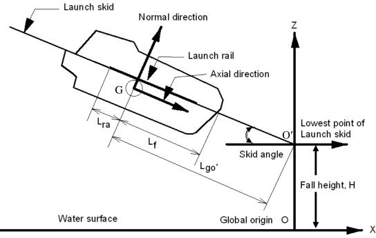
Fig. 1. Launch simulation of a free-fall lifeboat
