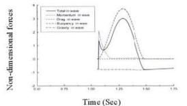
**Fig. 10b.** Non-dimensional forces at axial direction in wave ( $\theta$ =30°, H=1.75,  $\gamma$ =0.5m, T=2.0 sec,  $\phi = 0^{\circ}$ )
