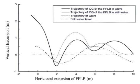
**Fig. 5.** Trajectory of CG of the FFLB in wave and in still water ( $\theta$ =30°, H=2.00,  $\gamma$ =0.5m, T=2.0 sec,  $\phi = 0^{\circ}$ )
