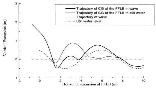
**Fig. 3.** Trajectory of CG of the FFLB in wave and in still water ( $\theta$ =30°, H=1.5m,  $\gamma$ =0.5m, T=2.0 sec,  $\phi = 0^{\circ}$ )
