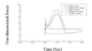
**Fig. 9b.** Non-dimensional forces at axial direction in wave ( $\theta$ =30°, H=1.5,  $\gamma$ =0.5m, T=2.0 sec,
