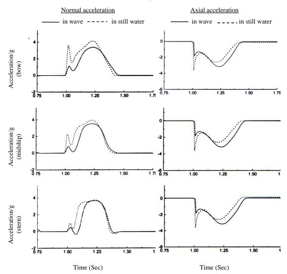
**Fig. 6.** Normal and axial acceleration of the boat at different positions in wave and in still water  $(\theta=30^\circ, H=1.5, \gamma=0.5\text{m}, T=2.0 \text{ sec}, \phi=0^\circ)$
