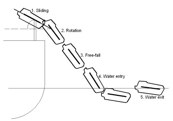
Fig. 2. Different phases of a free-fall lifeboat
