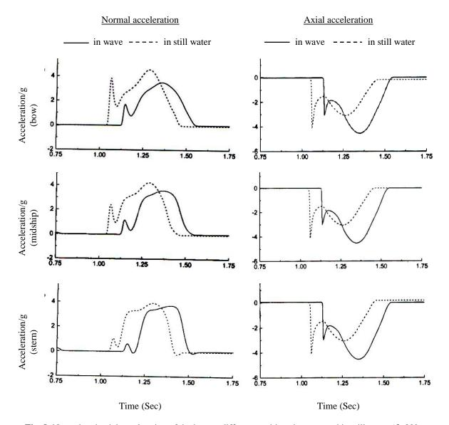
Fig. 8. Normal and axial acceleration of the boat at different positions in wave and in still water ( $\theta$ =30°, H=2.00,  $\gamma$ =0.5m, T=2.0 sec,  $\phi = 0^{\circ}$ )
