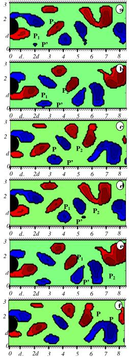
**Fig.3.** Coherent structures downstream the cylinder using  $\Gamma_2$  criterion for Re=159 with a time step of 0.16 T; from (a) to (f)
