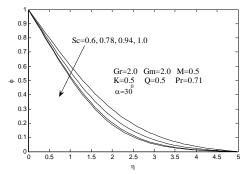
Fig.8. Effect of Sc on concentration profiles
