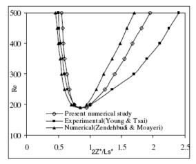
Fig. 4. Separation-reattachment curves for single restriction
