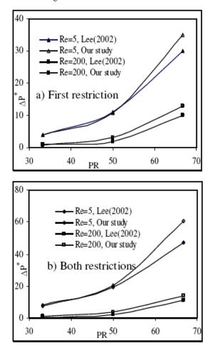
Fig. 3. Comparisons with the result of wall pressure drops across restrictions for Re=5 and 200 for PR=33.33%, 50% and 66.67%
