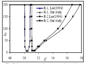
Fig. 5. Separation-reattachment curves for double restrictions
