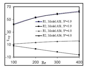
Fig. 10c. Variations of peak wall shear stress.
