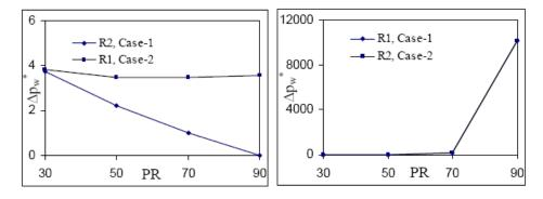
Fig. 7b. Variations of wall pressure drop at stenosis zone for Re=100 for case-1 and case-2.
