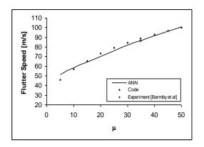
Fig. 7. Effect of wing/air mass ratio on flutter speed of model 73
