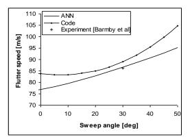
Fig. 6. Effect of sweep angle on flutter speed of model 73
