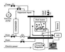
Fig. 1. A scheme of the experimental apparatus
