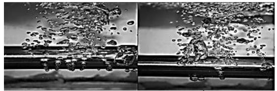
**Fig. 3.** Pool boiling of formic acid in 10 and 60kW.m<sup>-2</sup>
