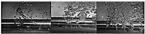
a) Heat flux 15kw/m
