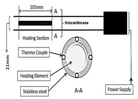
Fig. 2. Some details of heating section
