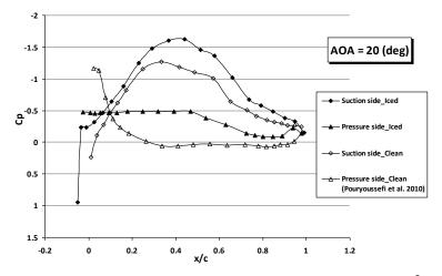
Fig. 6. The pressure coefficient distribution on the blade surface at 20  $^\circ$
