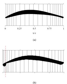
Fig. 4. The pressure taps locations on the surfaces of: (a) clean blade (Pouryoussefi *et al.* 2010); and (b) iced blade
