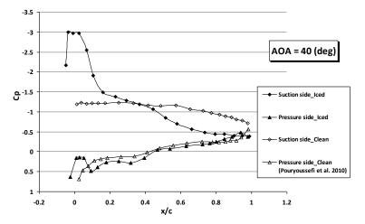
Fig. 10. The pressure coefficient distribution on the blade surface at 40  $^{\circ}$
