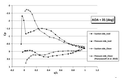
Fig. 9. The pressure coefficient distribution on the blade surface at 35  $^{\circ}$
