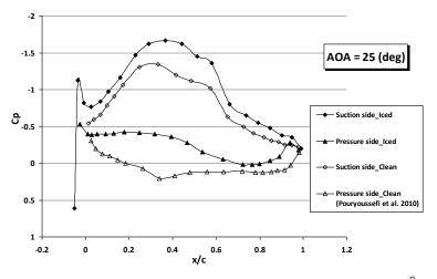
Fig. 7. The pressure coefficient distribution on the blade surface at 25  $^\circ$
