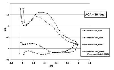
Fig. 8. The pressure coefficient distribution on the blade surface at  $30^{\circ}$
