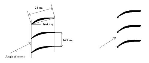
(a) (b) **Fig. 2.** Schematic view of the cascade of stator blades (experimental set-up in the wind tunnel): (a) clean blades (Pouryoussefi *et al.* 2010); and (b) iced blades
