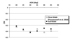
Fig. 14. The moment coefficient variation due to angle of attack changes
