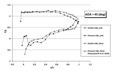
Fig. 11. The pressure coefficient distribution on the blade surface at 45  $^\circ$
