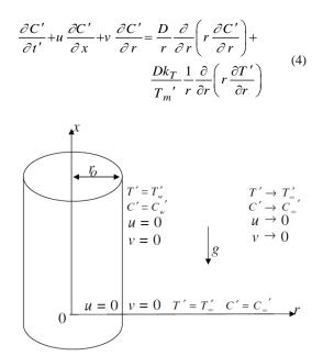
Fig. 1. Schematic of the investigated problem along with the boundary conditions, where the notations are defined in Nomenclature.
