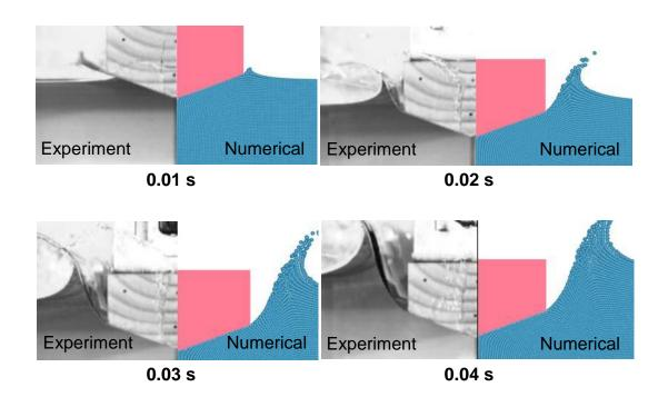
Fig. 10. Fluid flow, 1.64 kg impactor, 150 mm drop height,  $20^{\circ}$  deadrise angle
