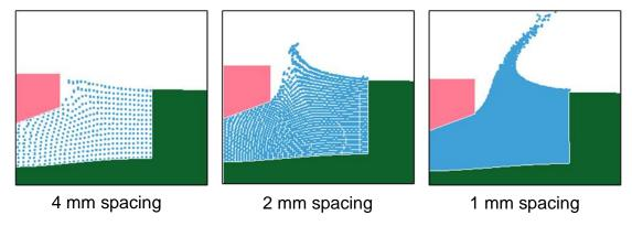
Fig. 5. Particle density investigation, fluid flow results.
