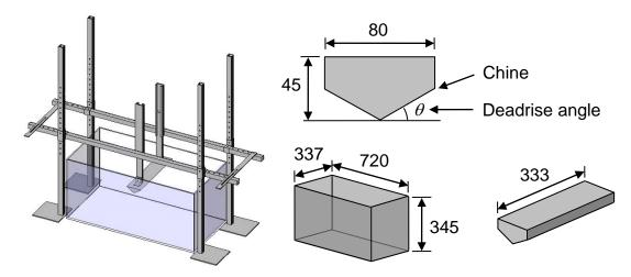
Fig. 1. Test rig and wedge specimen dimensions (mm).
