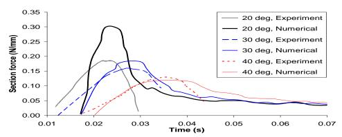
Fig. 13. Section force, 1.64 kg impactor, 150 mm drop height, varying deadrise angle.
