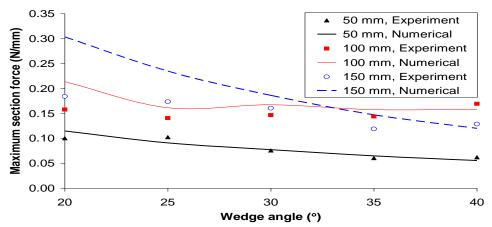
Fig. 7. Maximum section force, 1.64 kg impactor, varying drop height.
