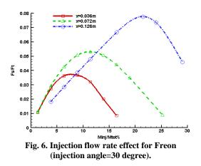
As the injection point gets off the throat, the optimized injection ratio increases. The reason for it is by getting off the throat, the area of the nozzle which is in contact with high pressure injecting liquid will be reduced and so to compensate this effect, more pressure should be applied on this surface. This could be done with increasing injection rate and create a strong shock.
