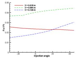
Fig. 12. Injection angle effect for three injection position, for N<sub>2</sub>O<sub>4</sub> fluid and m<sub>ini</sub>=0.5 kg/s.
