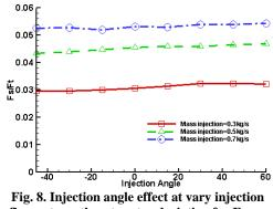
flow rate on thrust vector deviation for Freon  $(X_{inj} = 30\%$  Nozzle divergence length).
