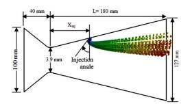
Fig. 3. Nozzle and injector geometrical parameters.
