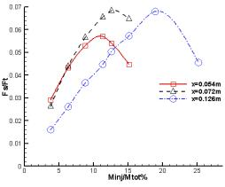
Fig. 7. Thrust vector variation for different injection flow rate for N<sub>2</sub>O<sub>4</sub> (Injection angle =30 degree).
