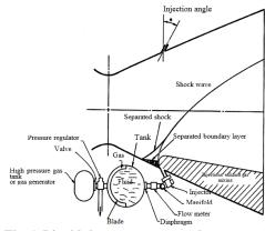
Fig. 1. Liquid thrust vector control system and its phenomena.
