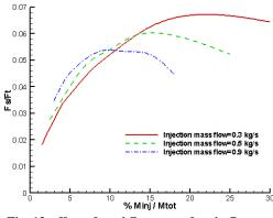
Fig. 13. effect of total flow rate of main flow on thrust vector deviation for Freon.
