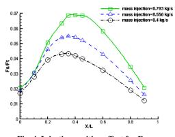
Fig. 4. Injection position effect for Freon (injection angle=30 degree).
