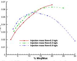
Fig. 14. Effect of total flow rate of main flow on thrust vector deviation for N<sub>2</sub>O<sub>4</sub>.
