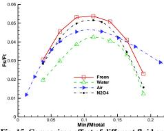
Fig. 15. Comparison effect of different fluid on thrust vector deviation.
