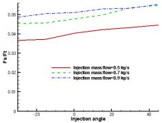
Fig. 11. Injection angle effect for three injection rate atX<sub>inj</sub>=0.054 m for N<sub>2</sub>O<sub>4</sub>.
