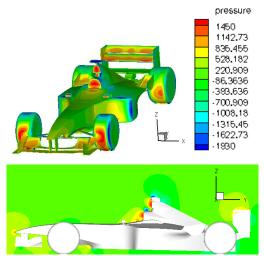
Fig. 13. Static pressure contours around and along the symmetry plane of the race car.
