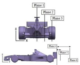
Fig. 3. Numerical simulation measurement planes.
