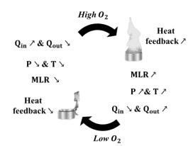
Fig. 4. Illustration of mechanisms leading to LF oscillations.
