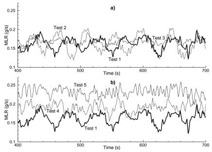
Fig. 12. MLR vs. time (a) for test cases 1 to 3, and (b) for test cases 1, 4 and 5.
