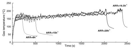
Fig. 7. Time evolution of gas temperature in the FE corner at a height of 0.95 m for different air renewal rates.
