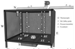
Fig. 1. Picture and schematic diagram of the experimental setup NYX showing instrumentation.
