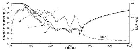
Fig. 9. Time evolution of oxygen mole fraction at different positions near the fuel pan (see Fig. 8 for the position of oxygen analyzers). For easier analysis, the MLR-time curve is superimposed on this figure.
