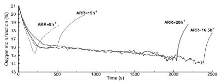
Fig. 6. Oxygen mole fraction in the lower part of the FE corner vs. time for different air renewal rates.
