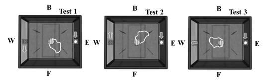
Fig. 11. Schematic diagrams showing the areas where the flame preferentially positioned for test cases 1 to 3 (top views).
