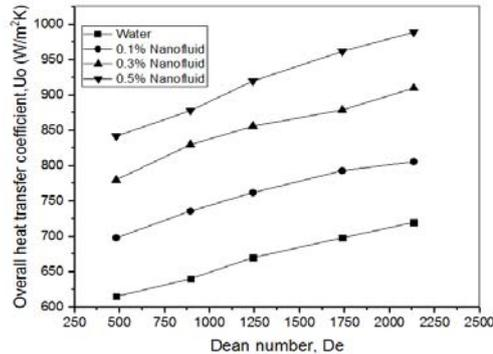
Fig. 5. Variation of overall heat transfer coefficient with tube side Dean number.
