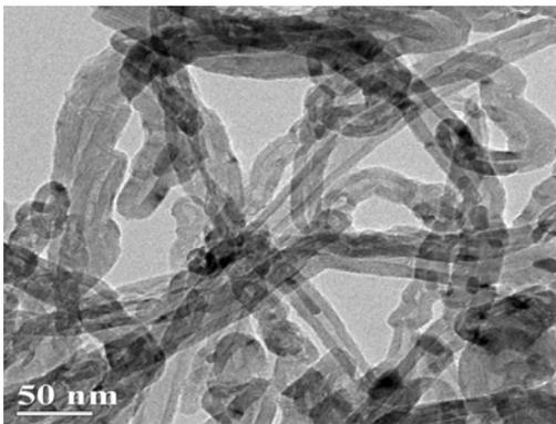
**Fig. 4. TEM image of MWCNT/water nanofluid.**
