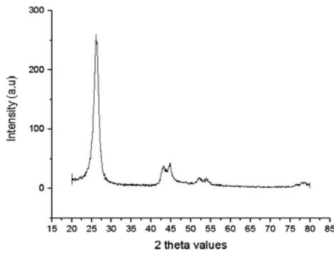
**Fig. 3. XRD pattern of MWCNT nanoparticle.**
