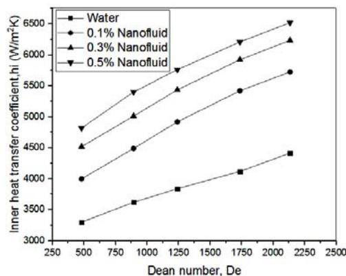
Fig. 6. Variation of inner heat transfer coefficient with tube side Dean number.
