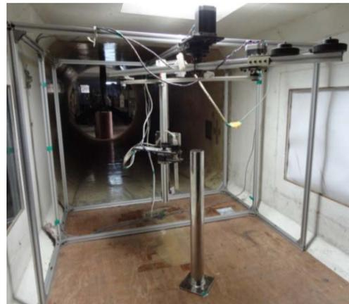
**Fig. 4. Tower model with traverse mechanism.**
