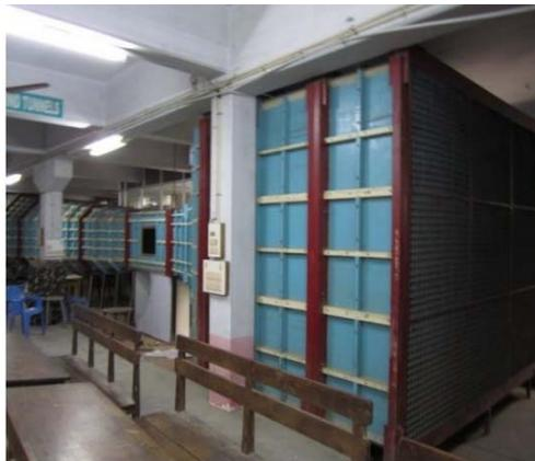
**Fig. 3. Low speed subsonic wind tunnel.**
