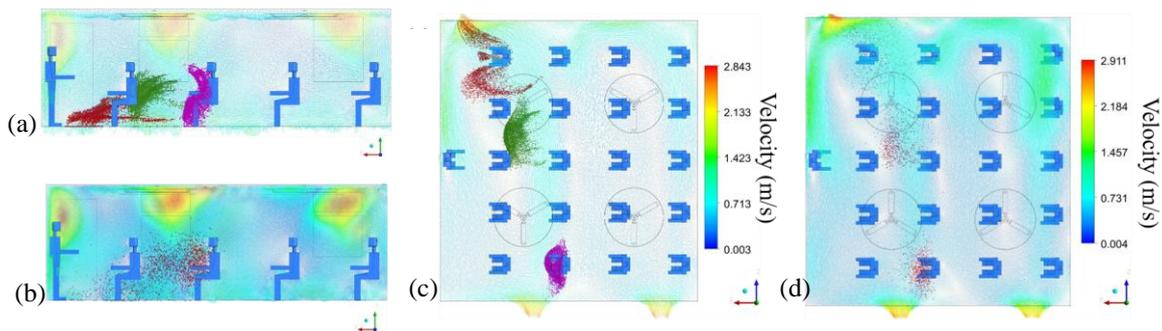
**Fig. 5** Students S6, S8, and S10 sneeze at 3.5 s with ceiling fans on (b), (d); ceiling fans off views (a) and (c). (a) and (b) show a lateral view with vectors on plane XY which split symmetrically the classroom. (c) and (d) depict a top view of the classroom, showing vectors on a plane aligned to XZ at the height of 1.20 m corresponding to the location of the student’s mouth from the floor
