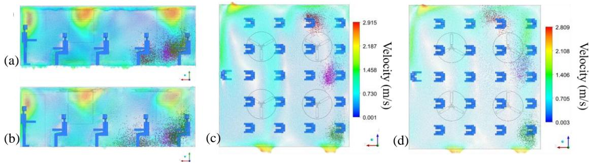
**Fig. 7** Students S16, S18, and S20 sneeze at 3.5 s with ceiling fans on (b), (d); ceiling fans off views (a) and (c). (a) and (b) show a lateral view with vectors on plane XY which split symmetrically the classroom. (c) and (d) depict a top view of the classroom, showing vectors on a plane aligned to XZ at the height of 1.20 m corresponding to the location of the student’s mouth from the floor
