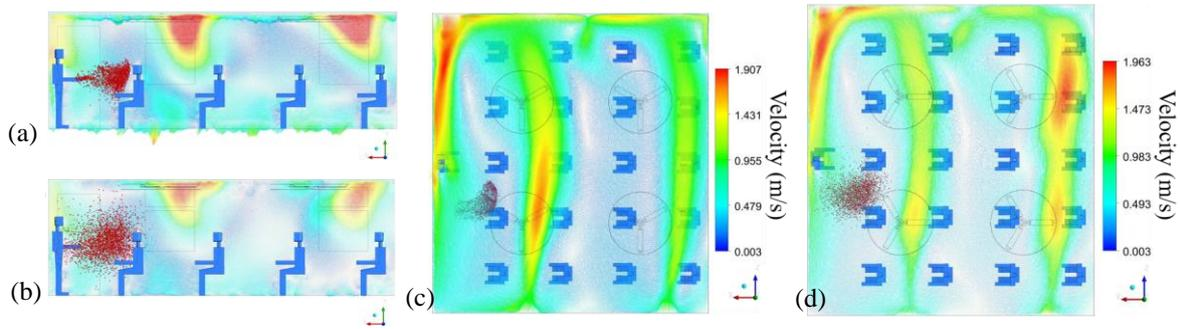
**Fig. 3** Teacher sneezes at 3.5 s with ceiling fans on (b), (d); ceiling fans off views (a) and (c). (a) and (b) show a lateral view with vectors on plane XY which split symmetrically the classroom. (c) and (d) depict a top view of the classroom, showing vectors on a plane aligned to XZ at the height of 1.20 m corresponding to the location of the student’s mouth from the floor
