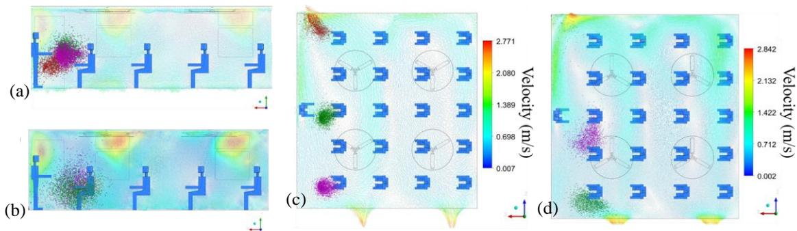
**Fig. 4** Students S1, S3 and S5 sneeze at 3.5 s with ceiling fans on (b), (d); ceiling fans off views (a) and (c). (a) and (b) show a lateral view with vectors on plane XY which split symmetrically the classroom. (c) and (d) depict a top view of the classroom, showing vectors on a plane aligned to XZ at the height of 1.20 m corresponding to the location of the student’s mouth from the floor
