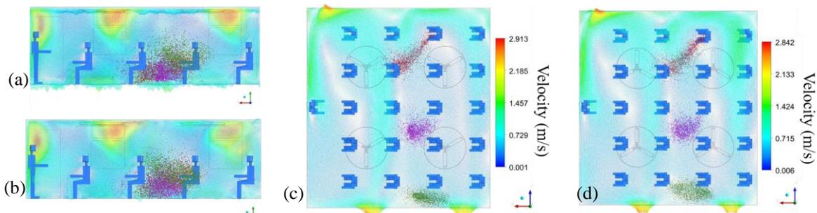
**Fig. 6** Students S11, S13, and S15 sneeze at 3.5 s with ceiling fans on (b), (d); ceiling fans off views (a) and (c). (a) and (b) show a lateral view with vectors on plane XY which split symmetrically the classroom. (c) and (d) depict a top view of the classroom, showing vectors on a plane aligned to XZ at the height of 1.20 m corresponding to the location of the student’s mouth from the floor
