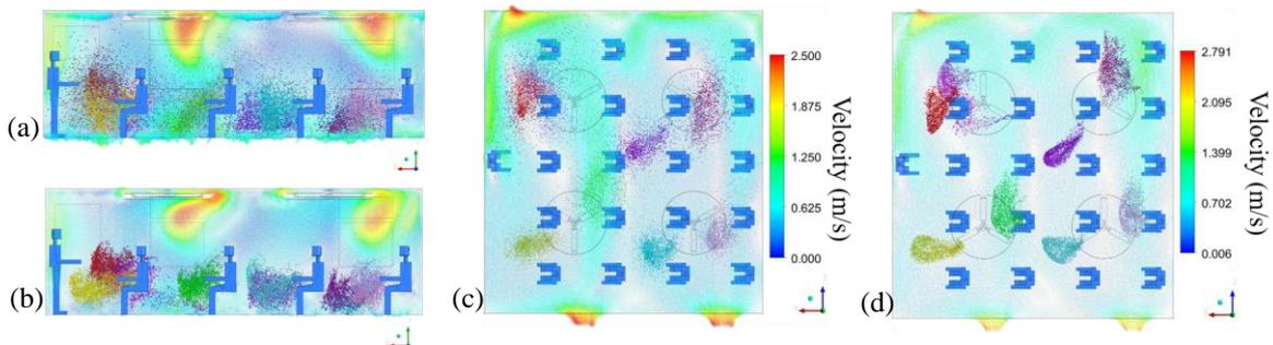
**Fig. 8** Students S2, S9, S12, S19, S4, S7, S14 and S17 sneeze at 3.5 s with ceiling fans on (b), (d); ceiling fans off views (a) and (c). (a) and (b) show a lateral view with vectors on plane XY which split symmetrically the classroom. (c) and (d) depict a top view of the classroom, showing vectors on a plane aligned to XZ at the height of 1.20 m corresponding to the location of the student’s mouth from the floor
