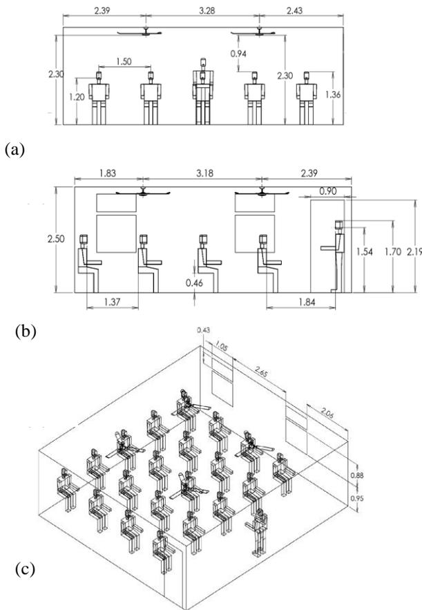
**Fig. 1 Classroom geometry and schematics. (a) Front view, (b) side view, and (c) isometric view. All numerical values are in meters**
