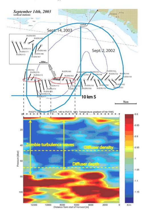
**Fig. 8 -** Contour plot of the Sept. 14, 2003 rms temperature dissipation rate for vertical profiles 7.5 km south of the diffuser. The Sept. 14, 2003 area of surface brightness anomalies is somewhat larger than that for Sept. 2, 2002.
