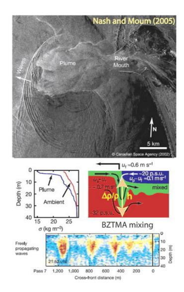
**Fig. 1b** - Formation of internal tidal waves at the Columbia River plume front, Nash and Moum (2005). The amplitude and speed  $c \approx \sqrt{g\rho'h}$  of the waves is determined by the density difference  $\rho' = \Delta\rho/\rho$  and penetration depth h of BZTMA mixing zone. Surface manifestations of the waves detected by the synthetic aperture radar (SAR) image at the top are transmitted near-vertically by small scale FTWs from turbulence produced by the solitons.
