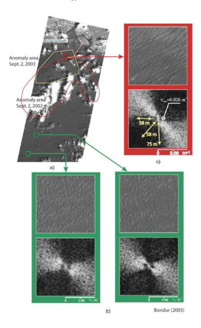
**Fig. 4 -** Surface brightness anomaly patterns from an Ikonos-2 optical image, Sept. 2, 2003, Bondur (2004). The strongest anomaly fragment (a) was found NW of the end of the diffuser pipe, with intense 38, 58 and 75 m wavelength Fourier components oriented EW, NE and N (double arrows) that are not present in background fragments (b). Anomaly areas for Sept. 2 observations in 2002 and 2003 are outlined. See Gibson *et al.* (2006) for the anomaly maps.
