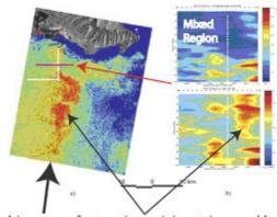
BZTMA chimneys of estuarine mixing, triggered by fossils of Sand Island outfall turbulence advected by alongshore tidal motions and strong offshore flows from Sept. 10 rains
