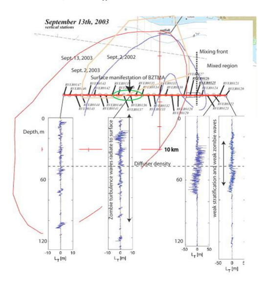
Fig. 11 - Vertical Thorpe overturn profiles at 5.5 km south of diffuser Sept. 13, 2004. Very large overturns  $L_{Tmax} > 30$  m to the east show weak stratification permits the growth of large zombie turbulence patches with weak radiation to the surface. Smaller 8 m zombie turbulence overturns to the west are somewhat larger than the original 6 m wastewater fossils and can effectively beam information to the surface about their presence in patterns of the 100-200 m BBL fossil waves.
