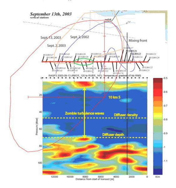
**Fig. 7** - Contour plot of the Sept. 13, 2003 rms temperature dissipation rate (as log  $(dT/dz)_{rms}$ ) for vertical profiles 5.5 km south of the diffuser. Active near surface regions of this indicator of fossil temperature turbulence are interpreted as evidence of breaking zombie turbulence waves (double arrows) above the wastewater trapping depth. The Sept. 13, 2003 area of surface brightness anomalies is about 200 km², ~ 4 times larger than that for Sept. 2, 2002.
