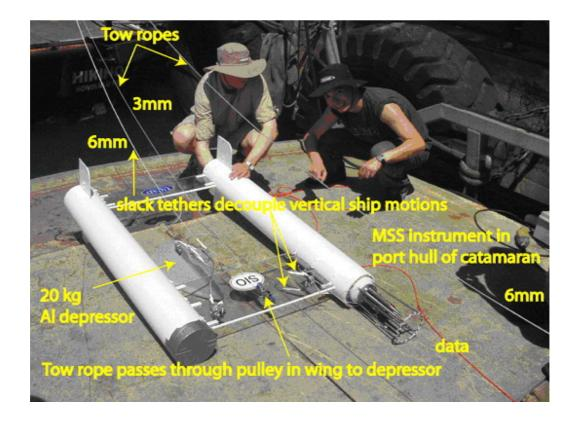
$\begin{tabular}{ll} \textbf{Fig. 13 - Catamaran tow body with MSS instrument mounted in port hull. Tow speeds of 2 m s$^{-1}$ exceeded the maximum speed permitted for shear sensors. Micro-temperature, micro-conductivity, micro-turbidity sensors and mean T, C and P sensors were operational. } \label{fig:conductivity}$
