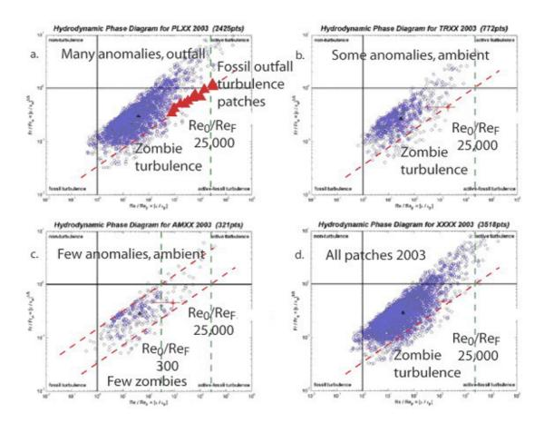
**Fig. 18** - Hydrodynamic phase diagrams for RASP 2003. The patch hydrodynamic state points have been sorted to detect any differences related to the ISINTECH brightness anomalies. Patches from the regions with strong anomalies, including the outfall, are shown in **a.** Regions with some anomalies but excluding the diffuser are shown in **b.** Regions with no anomalies and excluding the diffuser are shown in **c.** All regions are shown in **d.**
