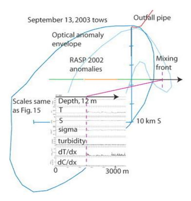
**Fig. 14** - Horizontal profiles Sept. 13, 2003, compared to sea surface brightness anomaly patterns (Figs. 5 and 7). A mixing front was detected at the indicated position outside the anomaly area, confirming the vertical profiles of Fig. 11 that suggest the BZTMA near-vertical internal waves (ZTWs) in the SE lobe have mixed away so much of the stratification that no more information can be transmitted near-vertically (Fig. 17).
