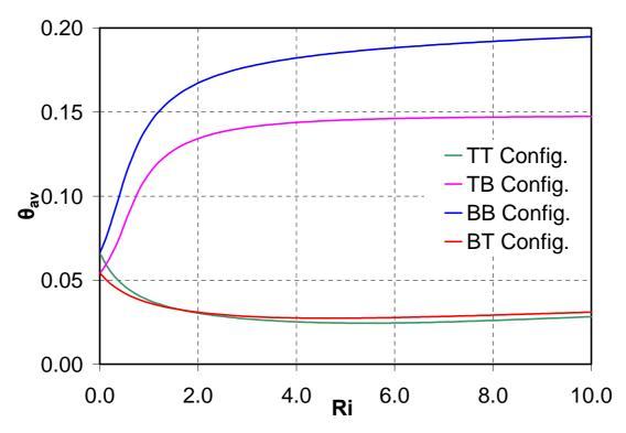
Fig. 9- Comparison of average bulk fluid temperature of the enclosure for different configurations
