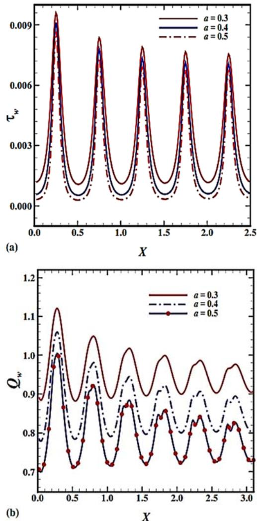
Fig. 3. (a) Skin friction and (b) Rate of heat transfer for  $a = 0.3, 0.4, 0.5$  while  $Pr = 7.0$ ,  $D_p = 10.0$ ,  $\gamma = 0.1$ ,  $\alpha_d = 0.1$  and  $\lambda = 1.0$ .
