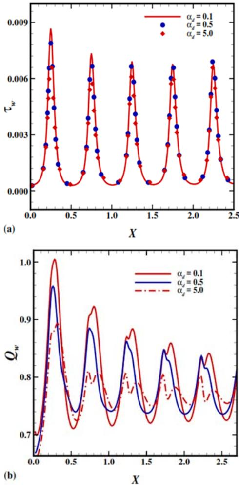
**Fig. 4. (a) Skin friction and (b) Rate of heat transfer for  $\alpha_d = 0.1, 1.0, 5.0$  while  $Pr = 7.0, D_p = 10.0, \gamma = 0.1, \lambda = 1.0$  and  $a = 0.5$ .**
