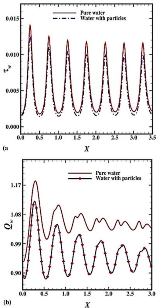
Fig. 2. (a) Skin friction and (b) Rate of heat transfer for  $D_p = 0.0, 10.0$  while  $Pr = 7.0$ ,  $\gamma = 0.1$ ,  $\alpha_d = 0.1$ ,  $\lambda = 1.0$  and  $a = 0.3$ .
