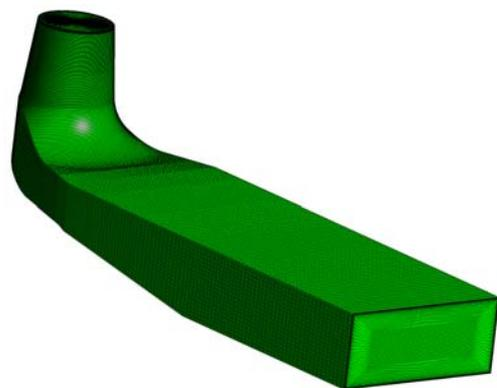
**Fig. 12. The generated mesh within the draft tube.**
