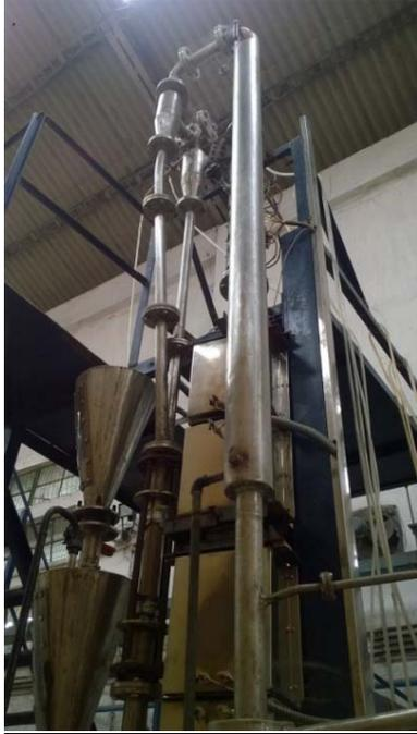
Fig. 1a. Pictorial view of CFB setup.
