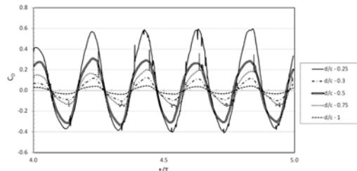
**Fig. 10. Variation of  $C_D$  at maximum  $C_L / C_D$  for various  $d/c$  ratio.**
