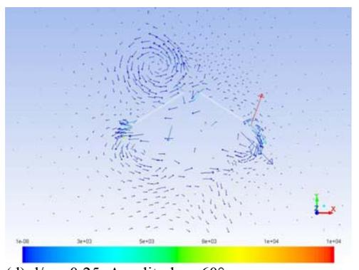
**Fig. 12. Vorticity vector representation of flappers for lowest values of  $\Delta C_L/\Delta C_D$ .**
