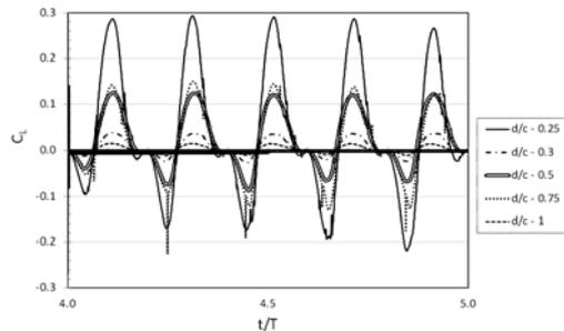
**Fig. 9. Variation of  $C_L$  at maximum  $C_L / C_D$  for various  $d/c$  ratio.**
