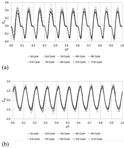
**Fig. 7. Convergence study of cycle: (a) lift Coefficient, and (b) drag coefficient at  $f = 10$  Hz and  $\theta_0 = 30^\circ$ .**
