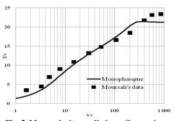
Fig. 5. Mean velocity predictions: Comparison with experimental results.
