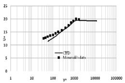
Fig. 8. Velocity profile plotted using the model (UL=1m/s; void fraction=1.5%): Comparison with experimental results.
