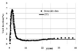
Fig. 9. Void fraction profile in vertical bubbly boundary layer: Comparison with the experimental data of Moursali *et al.* (1995) - (void fraction=0, 01).
