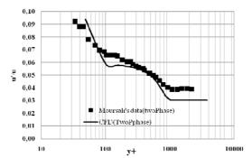
Fig. 10. Turbulent intensity profiles in vertical bubbly boundary layer. Comparison of the numerical results with the experimental data of Moursali *et al.* (1995)-(u=1m/s void fraction=0,015).
