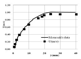
Fig. 4. Comparison of the liquid velocity profile with experimental results single phase flow.
