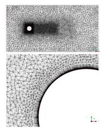
Fig. 2. 2D slice (Z=0 plane) of the mesh used for computations
