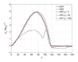
Fig. 10. Cf distribution [X03, X06 and X07]
