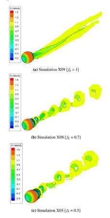
Fig. 15. Instantaneous vortical structures
