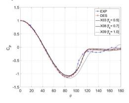
Fig. 12. C<sub>p</sub> distribution [X03, X08 and X09]
