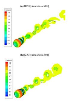
Fig. 7. Instantaneous vortical structures
