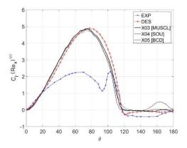
Fig. 6. Cf distribution [X03, X04 and X05]
