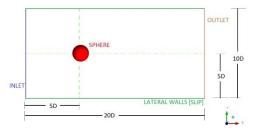
Fig. 1. Schematic of Computational Domain
