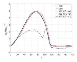
Fig. 4. Cf distribution [X01, X02 and X03]
