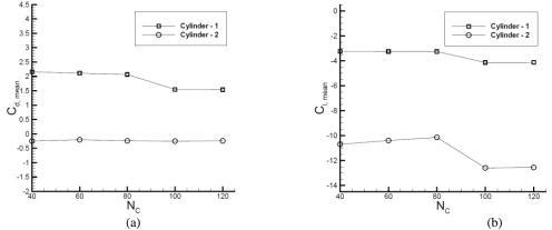
Fig. 3. Results of grid independence study (a) variation of drag coefficient (b) variation of lift coefficient, with increase in N<sub>c</sub>.
