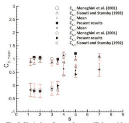
Fig. 8. Variation of mean drag coefficient with increase in inter-cylinder spacing for flow past two stationary tandem circular cylinders.
