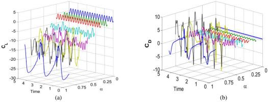
Fig. 10. Temporal variation of drag and lift coefficients for the downstream cylinder.
