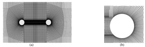
Fig. 2. (a) Schematic of grid mesh (b) magnified view of the mesh close to downstream cylinder.
