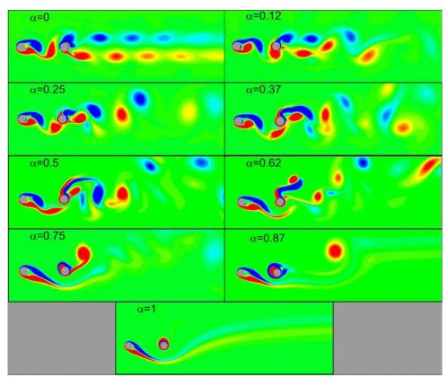
Fig. 9. Instantaneous vorticity contours for different values of.
