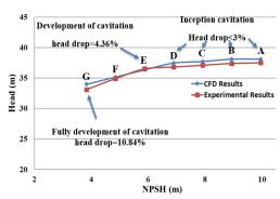
Fig. 7. NPSH for the cavitation characteristics prediction curve of the pump.
