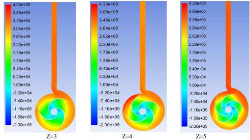
Fig. 8. Static pressure variations of the pump under different number of blades.
