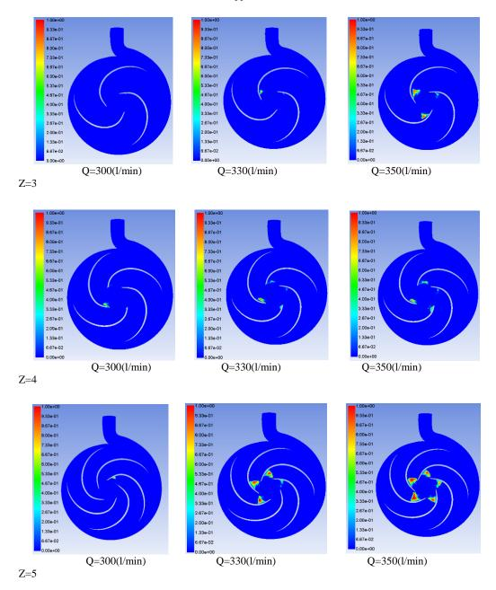
Fig. 16. Volume fraction distributions for the centrifugal pump under different number of impeller blades and flow rates.
