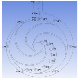
Fig. 10. Distribution of monitoring point's positions in the centrifugal pump.
