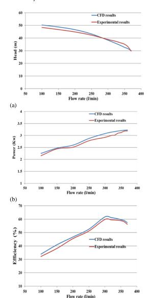
Fig. 6. Validation of the numerical and experimental (a) head, (b) power and (c) efficiency of the pump.
