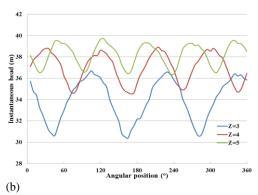
Fig. 14. Instantaneous head variations of centrifugal pump models having different number of blades (Z) under (a) single-phase and (b) cavitation conditions.
