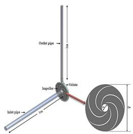
Fig. 4. Geometry of the centrifugal pump model.
