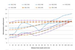
Fig. 23. Wall pressure distribution along the length of the duct.
