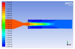
Fig. 13. Pressure contour for M = 2.5, NPR = 5and  $PCD = D_2$ .
