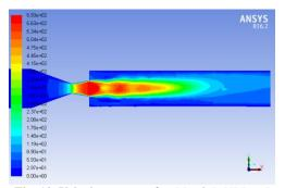
Fig. 10. Velocity contour for M = 2.5, NPR = 5 without control jets.
