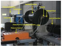
b) Experimental Setup Fig. 8. Experimental setup.
