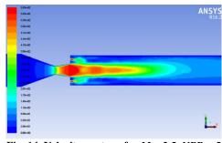
Fig. 14. Velocity contour for M = 2.5, NPR = 5and  $PCD = D_2$ .
