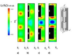
Fig. 10. Radial velocity profile: a) Smooth case (b'=0), b) case 2 (b'=0.25), c) case 4 (b'=0.5), and d) case 6 (b'=0.75). T=1.42. PIV results.
