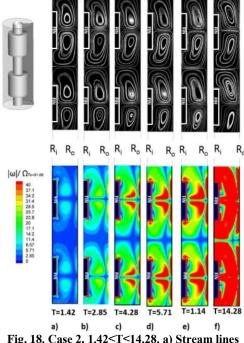
Fig. 18. Case 2, 1.42≤1≤14.28. a) Stream lines and b) vorticity magnitude. Numerical results.
