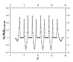
Fig. 17. Radial velocity profile along the whole system for case 4, T=5.71.
