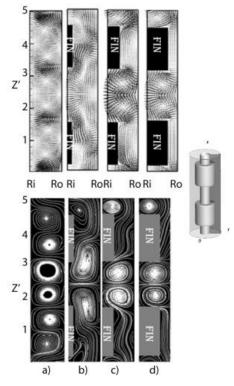
Fig. 8. Vortex pattern: vectors (high) and streamlines (low). a) Smooth case, b) case 2, c) case 4, and d) case 6. T=1.42. PIV results.
