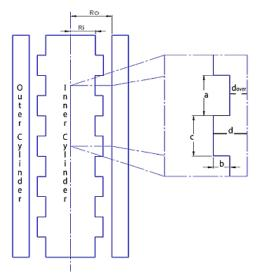
Fig. 1. Experimental setup. Outer cylinder radius ( $R_0$ ), inner cylinder radius (Ri), fin width (a), height fin (b), and length between fins (c).
