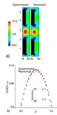
Fig. 4. Validation of the radial velocity profile, a) Case 4 (b'=0.5), Ta=81.68 and b) inward magnitude flow between fins.
