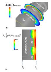
Fig. 11. Angular velocity (a) and pressure gradient (b), T=1.42, case 4. Numerical results.
