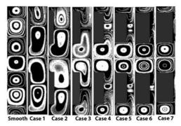
Fig. 9. Evolution of the vortex deformation (streamlines) for the geometric characteristics shown in Table 1. T=1.42. Numerical results.
