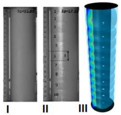
Fig. 6. KV results: (I) Smooth classic case on Couette flow, (II) Smooth case on Taylor vortex pattern (dimensions in centimeters). (III) 3D Numerical simulations on Taylor vortex pattern.
