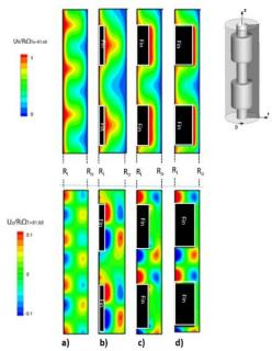
Fig. 12. Angular velocity (high) and axial velocity (low). a) Smooth case, b) case 2, c) case 4, and d) case 6. T=1.42. Numerical results.
