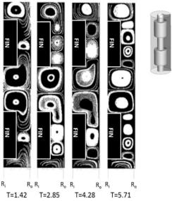
Fig. 15. Taylor number variation to case 4 (b'=0.5). Streamlines, 1.42≤T≤5.71. Numerical results.
