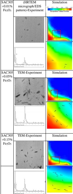
Fig. 11. Comparison of the Fe<sub>2</sub>O<sub>3</sub> nanoparticle distribution between simulation and experimental results.
