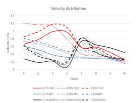
Fig. 13. Graph of velocity distribution of different types of nano-reinforced solder with different weighted percentages nanoparticles.
