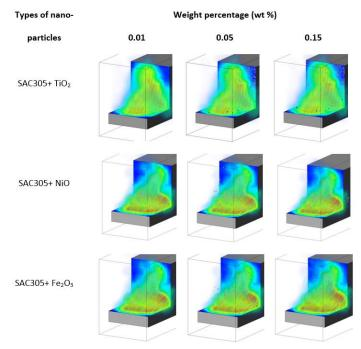
Fig. 7. 3D model-view of wetted SAC305 with nanoparticles.
