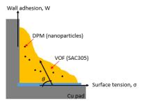
Fig. 5. Schematic diagram of boundary condition.
