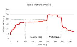
Fig. 1. Thermal profile.
