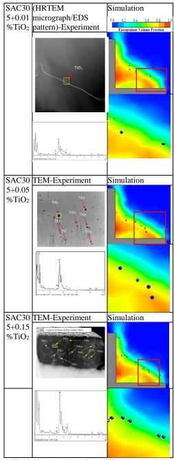
Fig. 9. Comparison of the TiO<sub>2</sub> nanoparticle distribution between simulation and experimental results.
