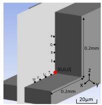
Fig. 12. Specified points near the base metal and the terminal of 01005 capacitor (ultra-fine package).
