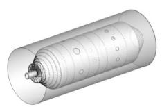
Fig. 4. Combustor model.
