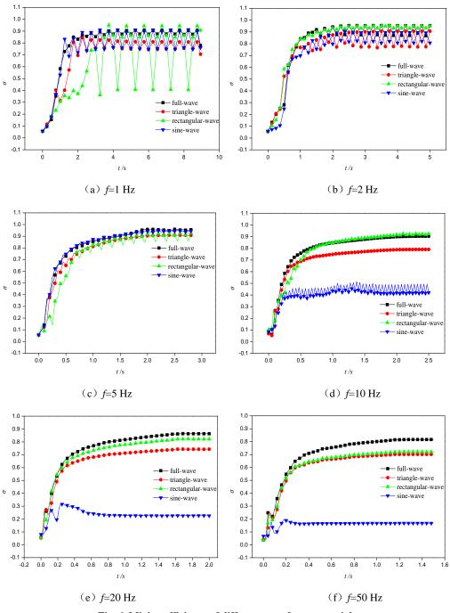
Fig. 6. Mixing efficiency of different waveform potentials.
