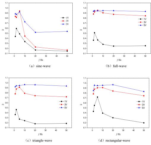
Fig. 7. Variation of mixing efficiency with frequency at different voltages.
