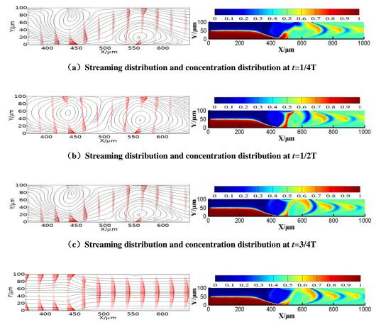
(d) Streaming distribution and concentration distribution at *t*=1T Fig. 5. Streaming distribution and concentration distribution in one triangular waveform at *V*<sub>0</sub>=3 V and *f*=5 Hz.
