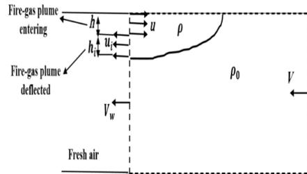
Fig. 4. Control volume of calculating the boundary condition at one-dimensional zone.
