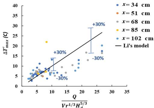
**Fig. 10. Comparison between experimental maximum temperature rise results of this study and the proposed model by *Li et al.* for different fire source locations**
