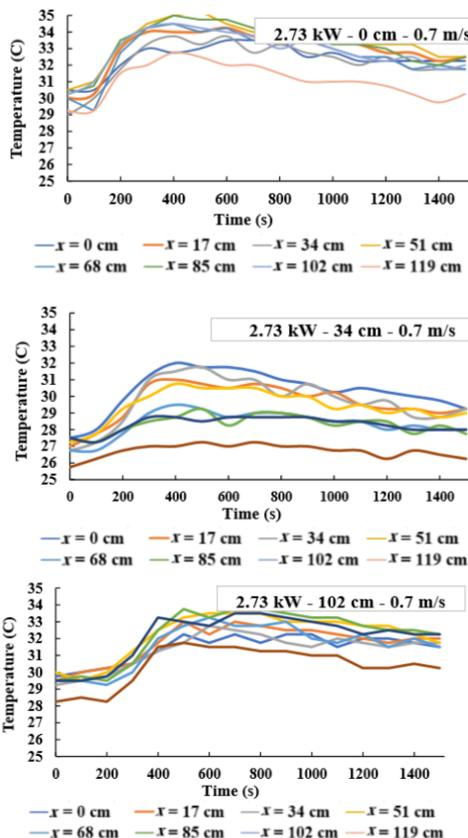
Fig. 6. Temperature profile of 2.73 kW fire at 0.7 m/s for different fire source locations.
