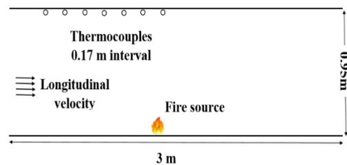
Fig. 1. Scaled tunnel drawing.
