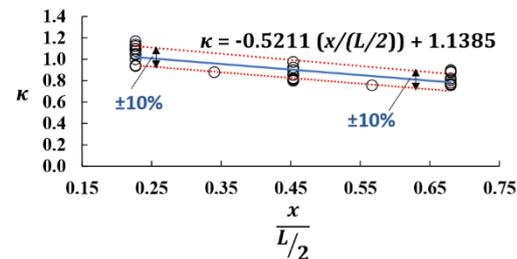
**Fig. 11. Correlation of correction factor  $\kappa$  with dimensionless distance  $x/(L/2)$ .**
