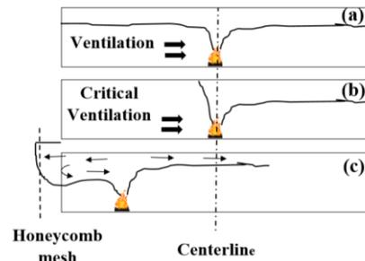
Fig. 5. Schematic view of smoke flow a) with the ventilation velocity smaller than the critical velocity, b) under the critical velocity, and c) when the distance between the fire source and the fan is reduced.
