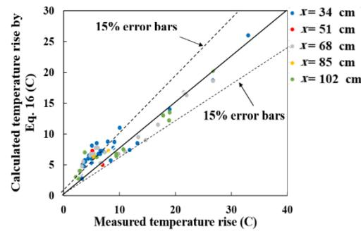
**Fig. 12. Comparison between experimentally measured and calculated maximum thermal smoke temperature rises.**
