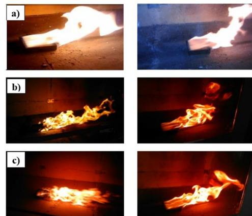
Fig. 8. Pictures of flame shape for two different scenarios: a) fire source at the origin, b) and c) fire source in a place other than the origin.
