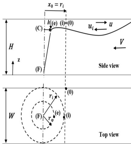
Fig. 3. Fire plume schematic view.
