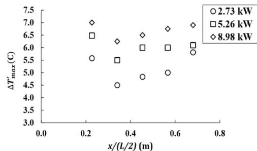
Fig. 9. Maximum temperature rise versus various dimensionless longitudinal fire locations.
