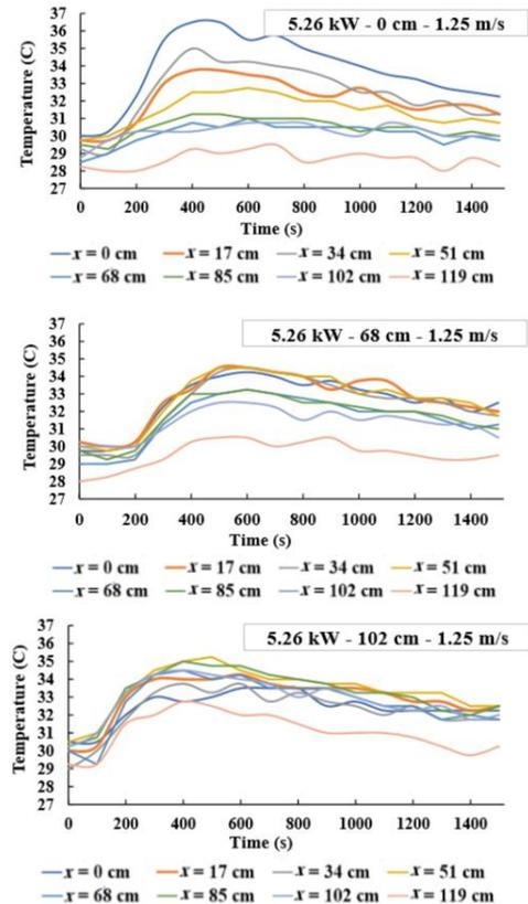
Fig. 7. Temperature profile of 5.26 kW fire at 1.25 m/s for different fire source locations.
