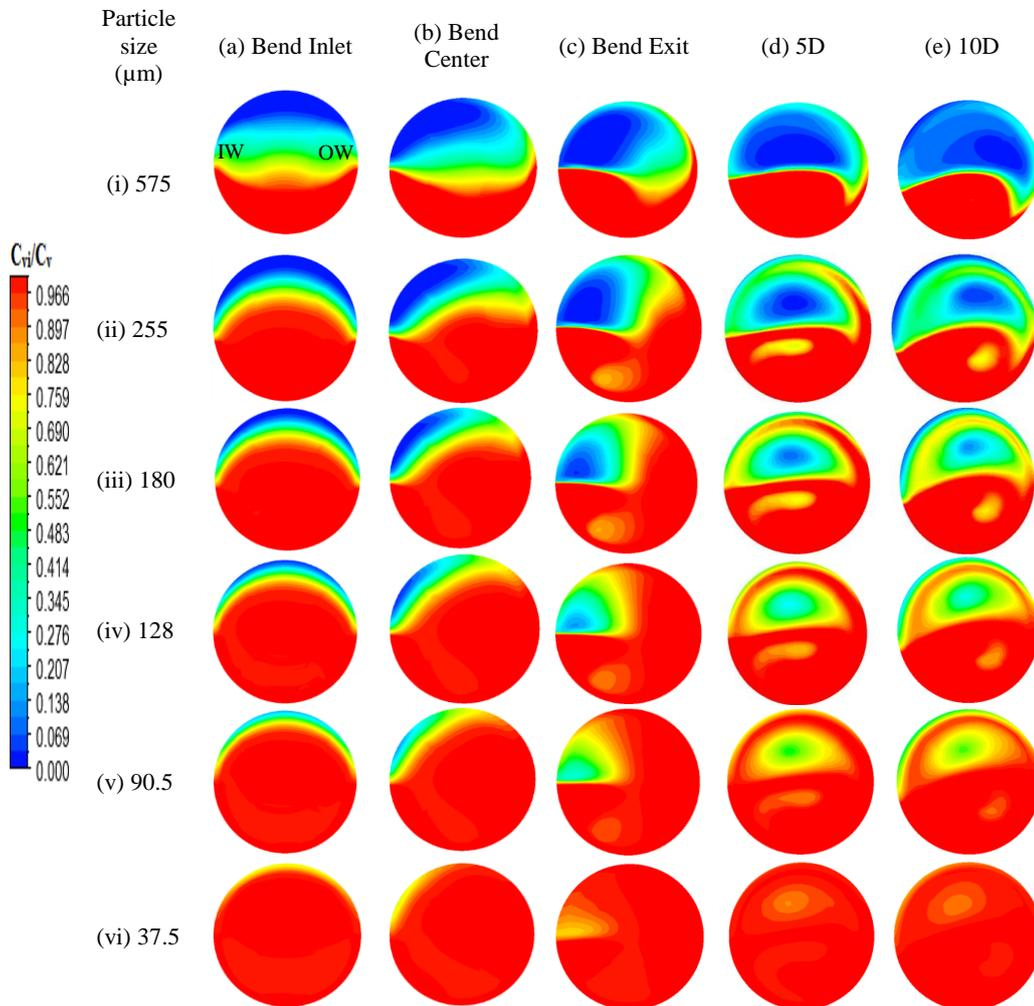
**Fig. 6 Cross-sectional normalized concentration contours (outer wall at right side) of each size particles at different angular positions, 5D, 10D distances from bend exit at velocity = 2.25 m/s,  $C_w = 9.82\%$ .**
