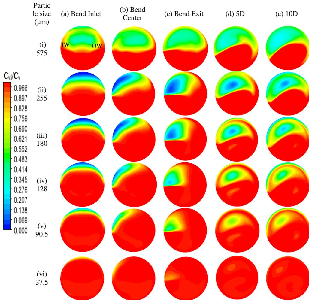
**Fig. 8** Cross-sectional normalized concentration contours (outer wall at right side) of each size particles at different angular positions, 5D, 10D distances from bend exit at velocity = 2.25 m/s,  $C_w = 44.26\%$ .
