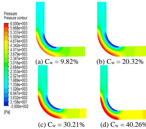
**Fig. 5. Absolute pressure variation with the solid concentration in pipe bend at the mid horizontal plane at  $V=3.5$  m/s.**
