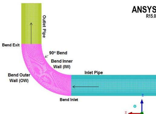
(b) Enlarged view of mesh in the pipe bend
