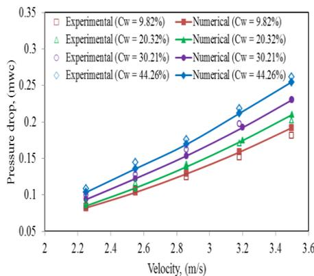
**Fig. 3. Comparison of predicted pressure drop to the experimental results of Mishra *et al.* (1998a) for different weighted solid concentration and velocity.**
