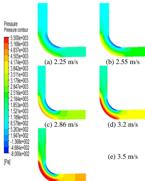
**Fig. 4. Absolute pressure variation with flow velocity in pipe bend at the mid horizontal plane at  $C_w = 44.26\%$ .**
