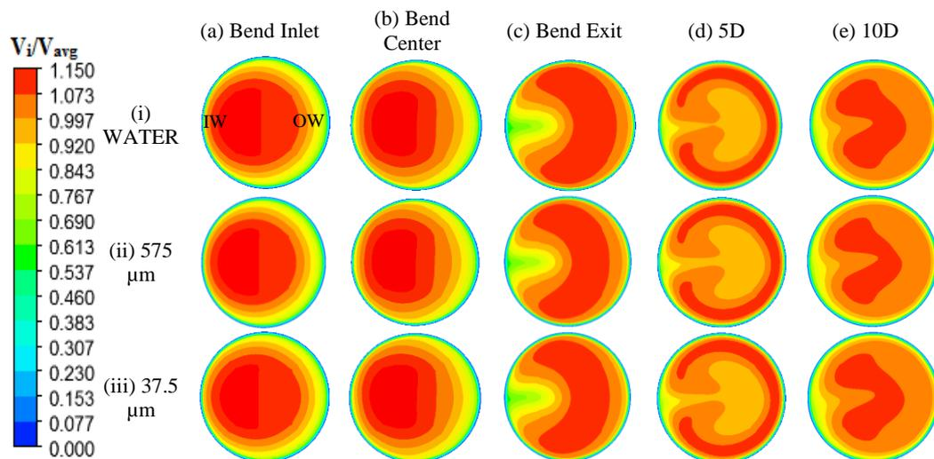
**Fig. 9** Cross-sectional normalized velocity contours (outer wall at right side) for water, particle size of 575 μm and 37.5 μm at different angular positions, 5D, 10D distances from bend exit at velocity = 3.5 m/s,  $C_w = 9.82\%$ .
