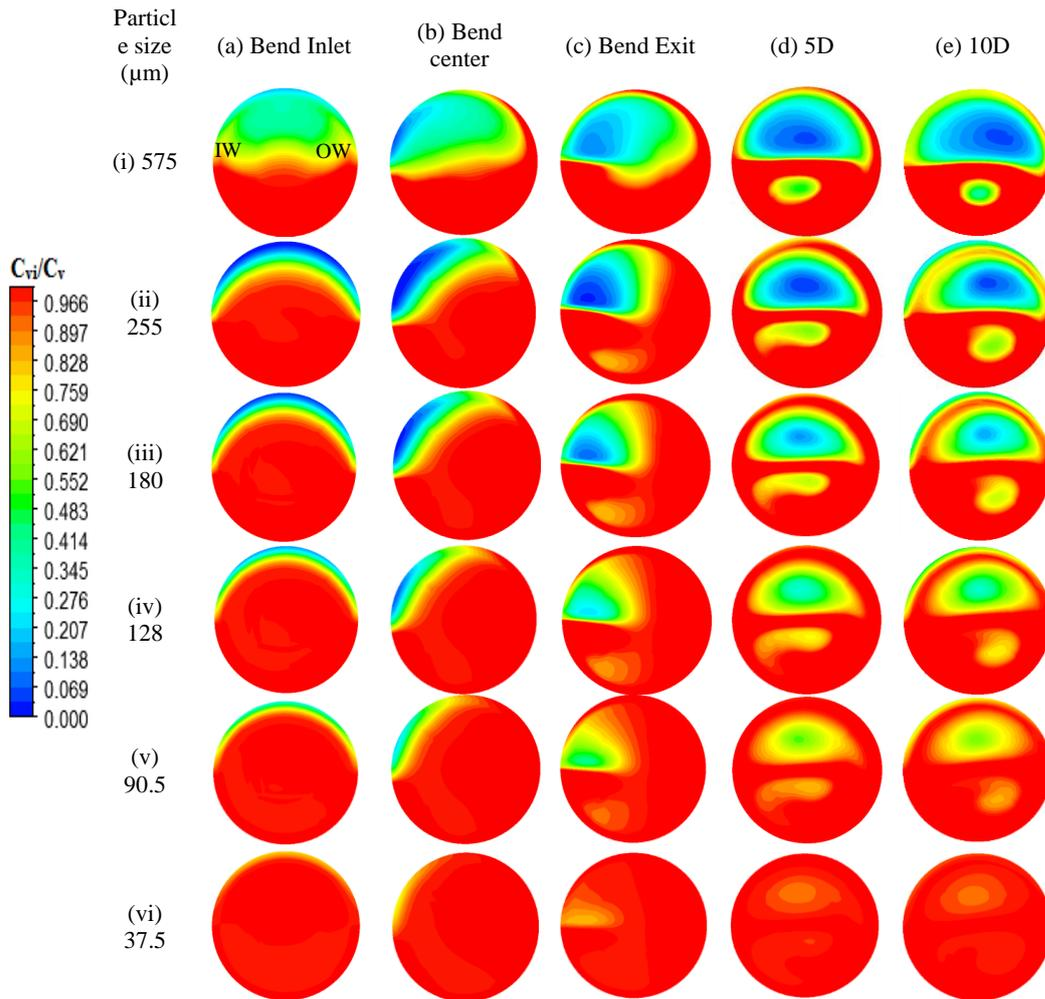
**Fig. 7** Cross-sectional normalized concentration contours (outer wall at right side) of each size particles at different angular positions, 5D, 10D distances from bend exit at velocity = 3.5 m/s,  $C_w = 9.82\%$ .
