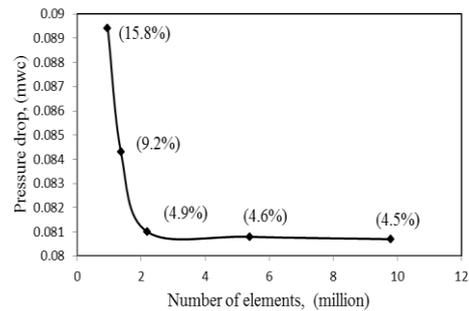
**Fig. 2. Pressure drop variation with the number of mesh elements.**
