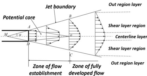
Fig. 6. Schematic of the turbulent round free jet.
