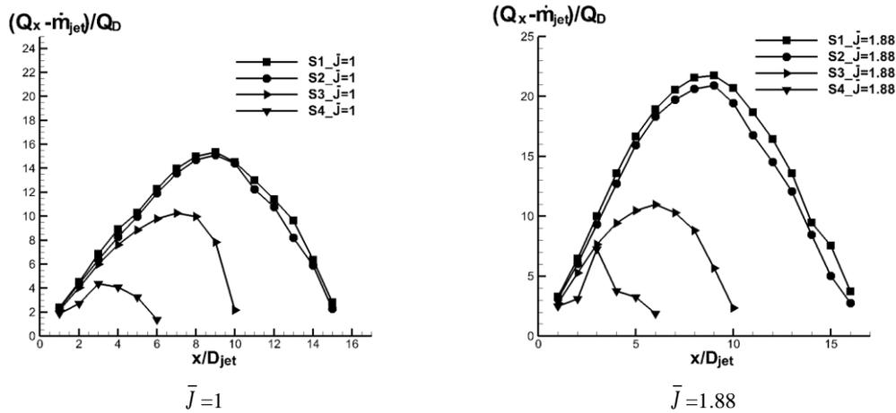
Fig. 11. Normalized entrainment rates of the surrounding gas into the jet along the axial direction at  $T=0.005s$ .
