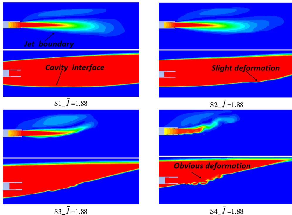
Fig. 8. As the relative position varies, jet boundary and cavity interface interaction are shown at  $T=0.005s$ .
