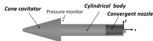
Fig. 9. Physical model of simulation.
