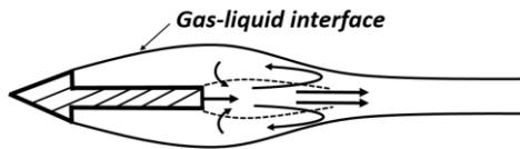
Fig. 4. Structure of the cavity closure onto a central jet of  $\bar{P} > 1$
