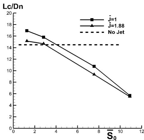
**Fig. 6.** Dimensionless cavity length as the distance parameter varies.
