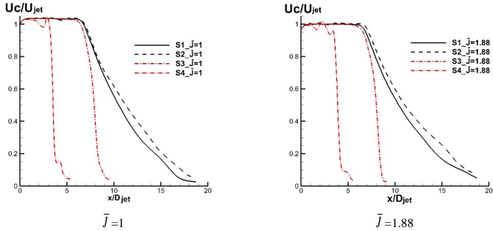
Fig. 10. Normalized centerline axial mean velocity decay at  $T=0.005s$ .
