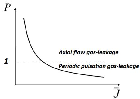
Fig. 3. Improved criterion for the cavity gas-leakage pattern under jet effects.
