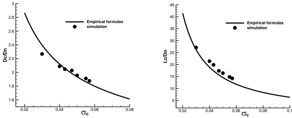
Fig. 1. Dimensionless maximum diameter and length of the cavity at different cavitation number.
