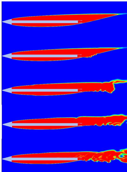
Fig. 4. Cavity interface evolution when  $\bar{P} < 1$  and  $\bar{S}_0 < L_2/D_n$ .
