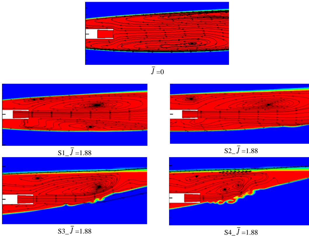
**Fig. 9.** As the relative position varies , the velocity streamline inside the cavity is showed at  $T=0.005s$ .
