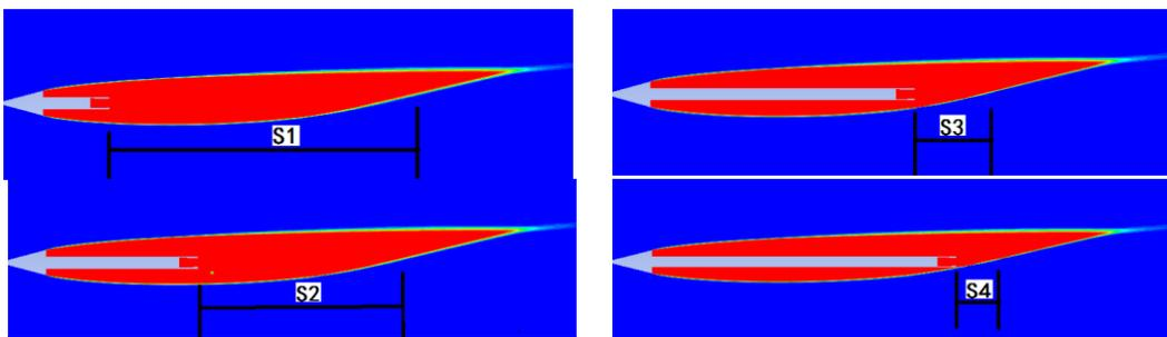
Fig. 2. Relative position between nozzle exit and cavity.
