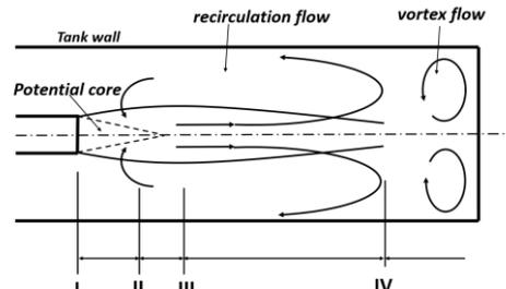
Fig. 7. Schematic of the turbulent round confined jet.
