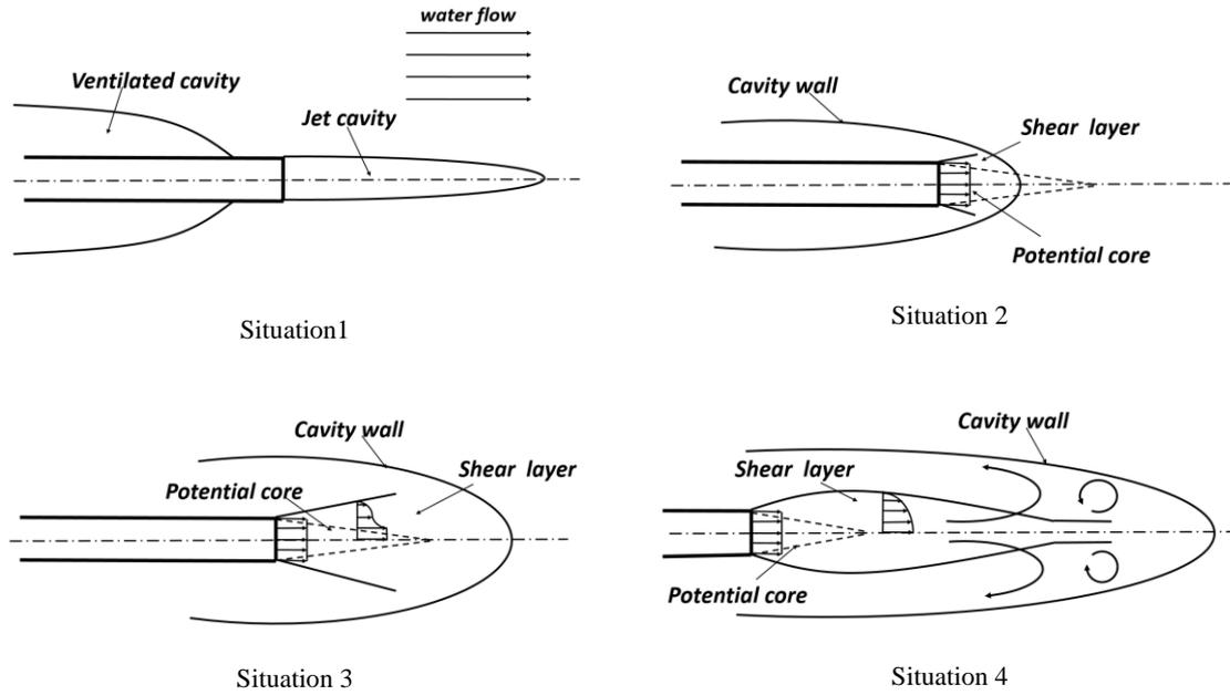
**Fig.8. Criterion for the jet/cavity interaction mechanism of varying relative position.**
