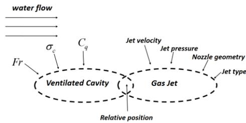
Fig. 1. Key parameters in the jet/cavity interaction.
