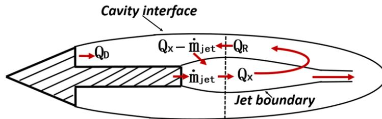
Fig. 21. Schematic of the cavity internal flow structure with a gas jet.
