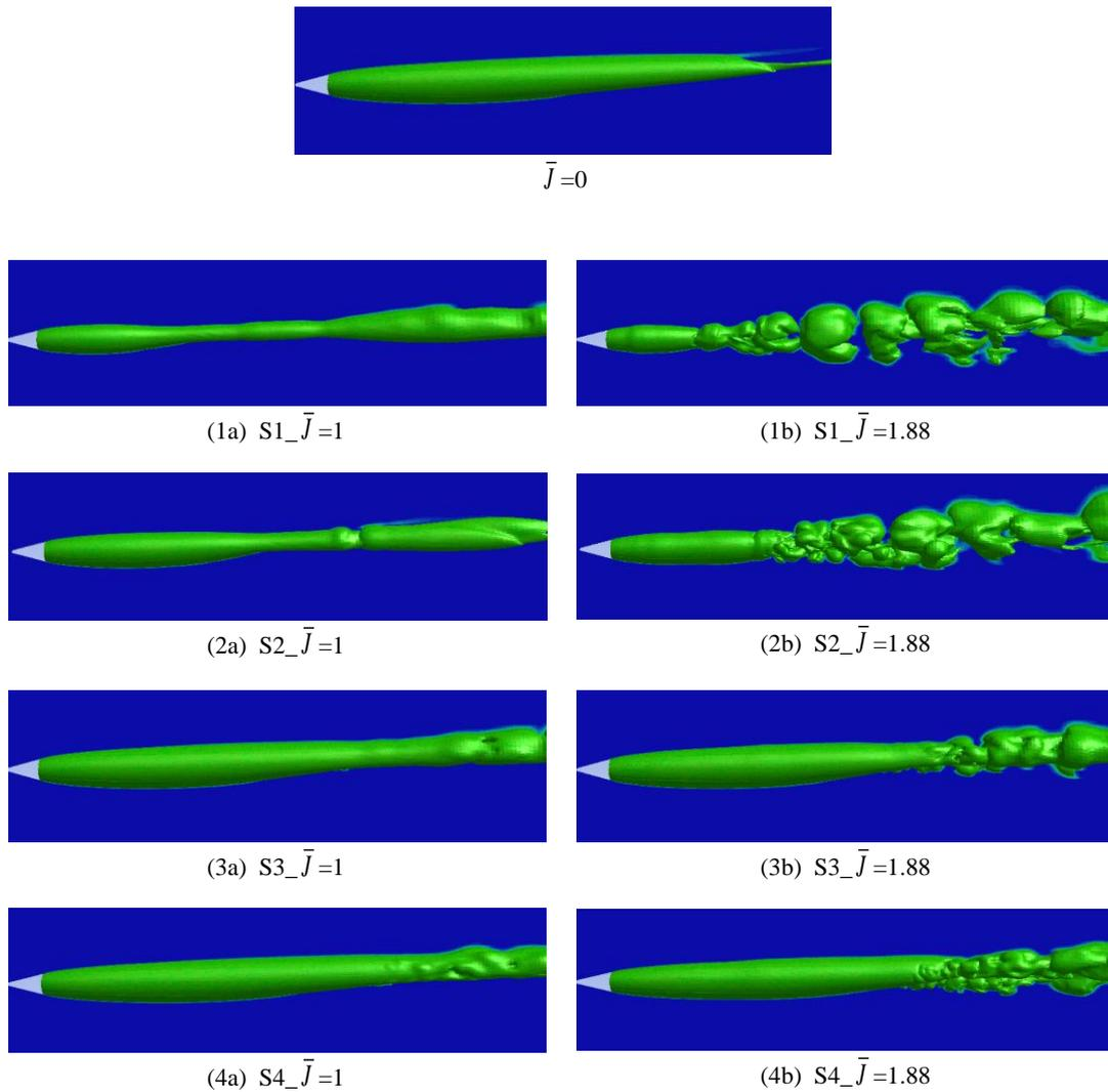
**Fig. 5.** Cavity morphology characteristics for varying relative position and jet strength at  $T=0.15s$ . The cavity interface is obtained by gas volume fraction of 0.5. Left :  $\bar{P} > 1$  and right :  $\bar{P} < 1$ .
