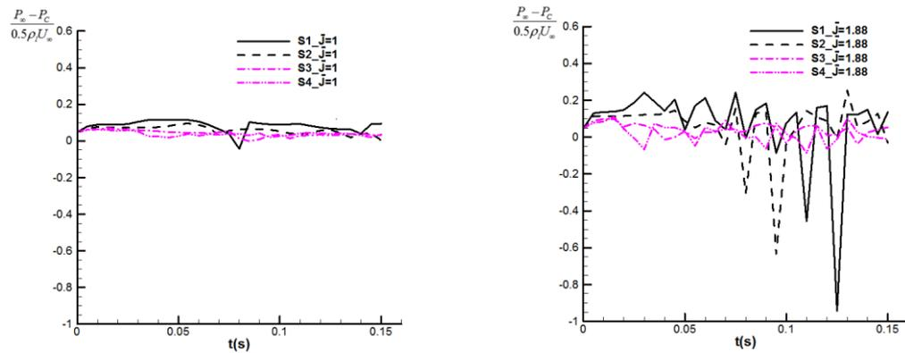
Fig. 7. Pressure pulsation characteristics inside the cavity for different relative position and jet strength.
