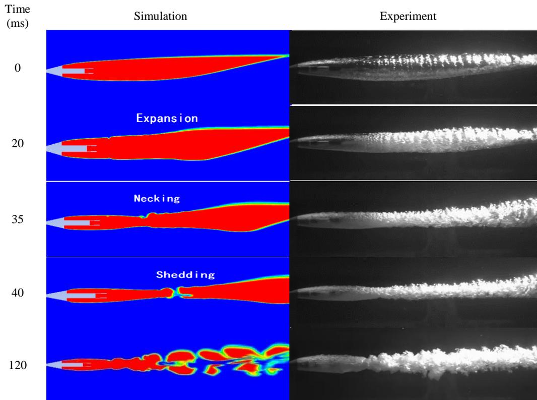
Fig. 3. Cavity interface evolution showed by the contours of volume fraction when  $\bar{P} < 1$  and  $\bar{S}_0 > L_2/D_n$  (blue regions: water, red regions: gas).
