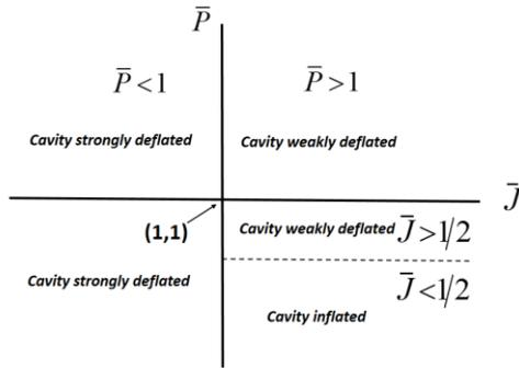
Fig. 2. Criterion for the jet/cavity closure interaction mechanism by Paryshev and Money.
