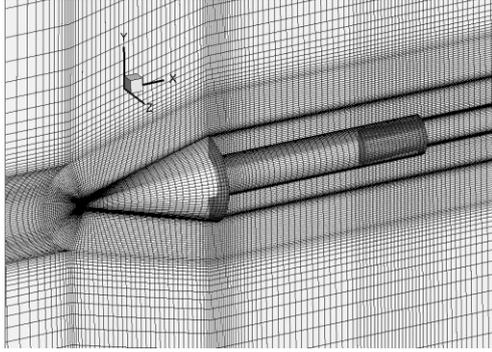
**Fig. 10. The computational mesh.**
