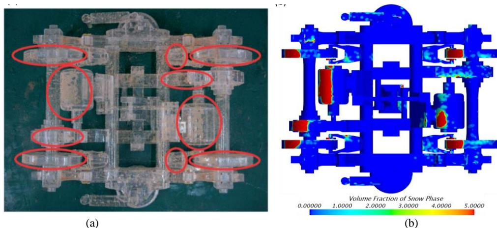
**Fig. 10. Comparison of experiment and numerical simulation: (a) Particle accumulation of tunnel experiment; Gao *et al.* (2018a). (b) Particle accumulation of numerical simulation.**
