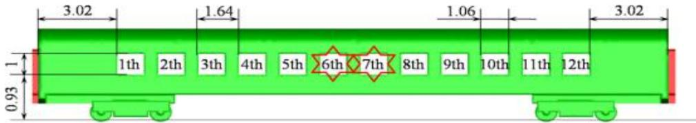
Fig. 2. Details of the windows on the second passenger car (m).
