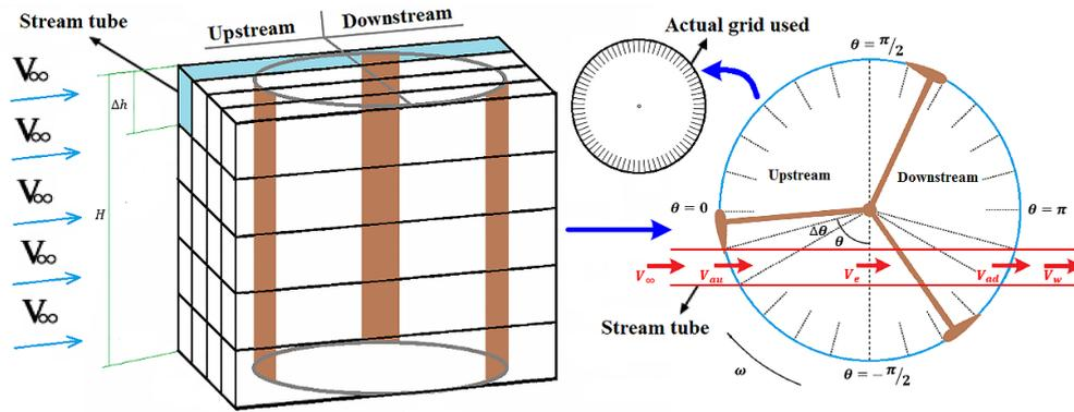
Fig. 3. Sketch of space division for DMST model developed in Darrieus VAWTs.
