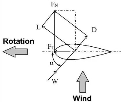
**Fig. 2. The aerodynamic force components influencing airfoil section.**
