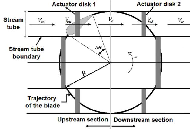
Fig. 1. Sketch of upstream and downstream section in DMST model.
