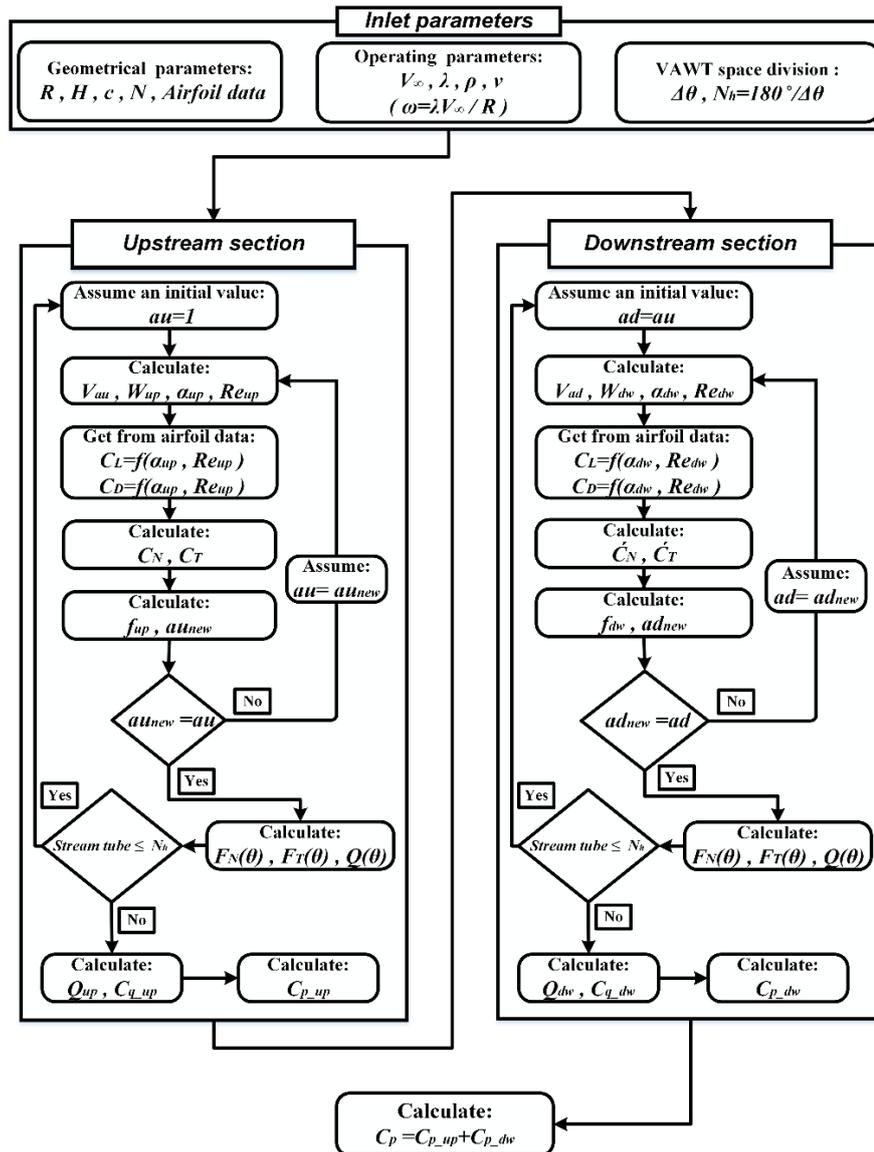
Fig. 4. Flowchart of DMST model developed for performance prediction of Darrieus VAWTs.
