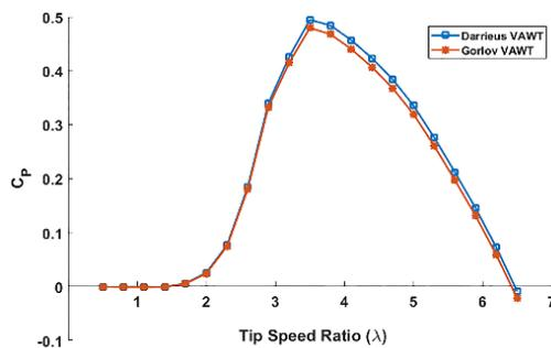
**Fig. 9. Comparing aerodynamic performance ( $C_p$ ) of Gorlov and Darrieus VAWTs.**
