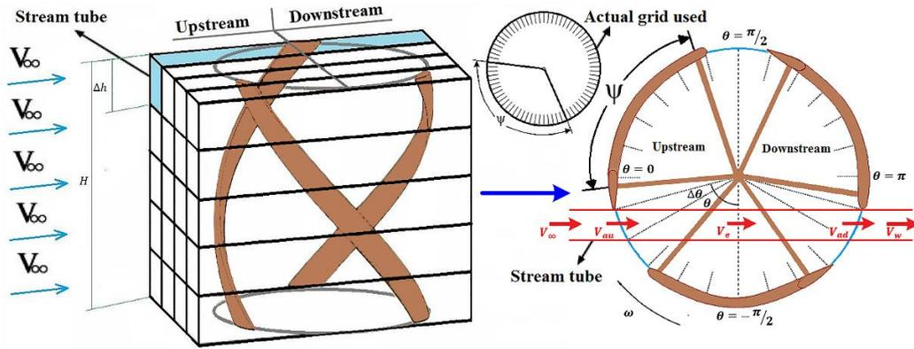
Fig. 6. Sketch of space division for DMST model developed in Gorlov VAWTs.
