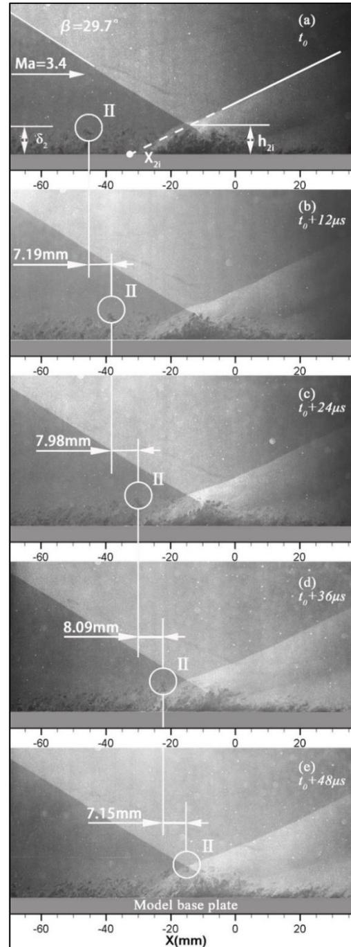
Fig. 7. NPLS images of SWTBLI in streamwise plane ( $\delta_2=0.72\delta$ ).
