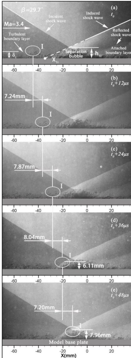
Fig. 6. NPLS images of SWTBLI in streamwise plane ( $\delta_1=0.55\delta$ ).
