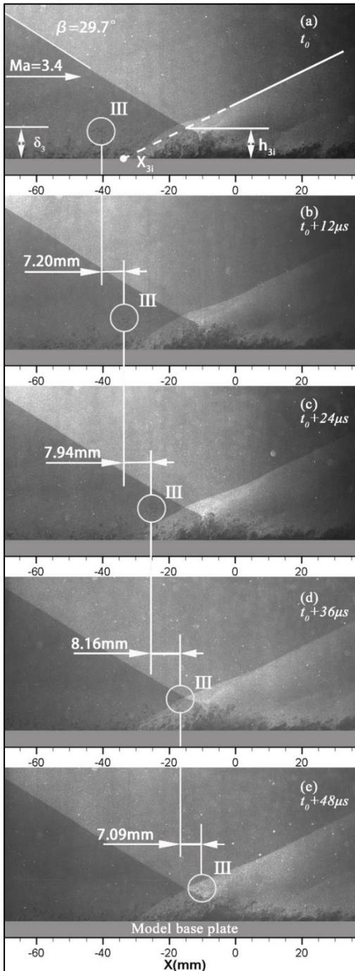
**Fig. 8. NPLS images of SWTBLI in streamwise plane ( $\delta_3=0.87\delta$ ).**
