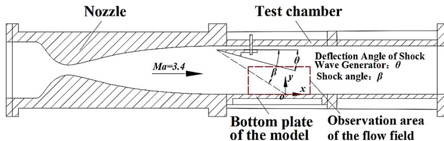
Fig. 2. Schematic of model installation.
