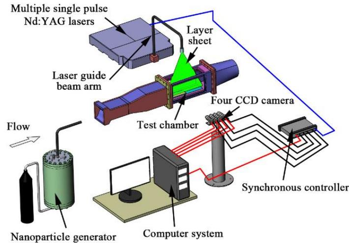
**Fig. 3. Schematic of NPLS system.**
