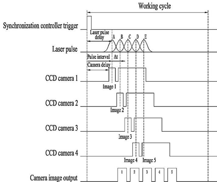
Fig. 5. Working timing diagram of NPLS system.
