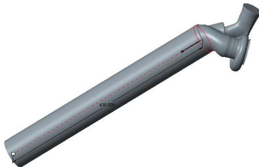
Fig. 5. Turbine housing model with extended outlet.
