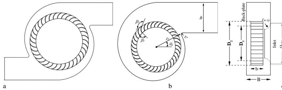
**Fig. 5. A schematic of front view of (a) double outlet, (b) single outlet squirrel cage fans, and (c) side view of a single outlet type with the dimensions.**
