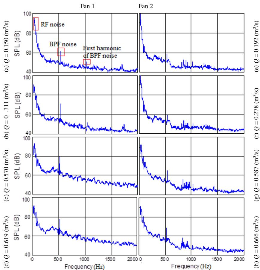
**Fig. 11.** Frequency spectra of SPL at the outlet channel of fan 1 (lower outlet) and 2.
