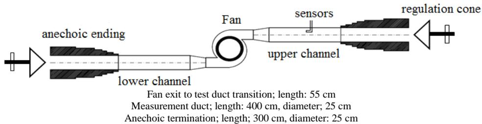
**Fig. 6. A schematic of the test installation (sensors are microphone, Pitot tube, and thermometer).**
