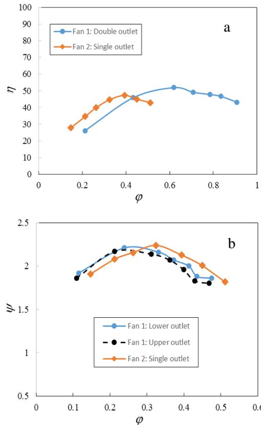
**Fig. 9.** Variations of (a) efficiency and (b) total pressure coefficient, versus traditional flow coefficient.
