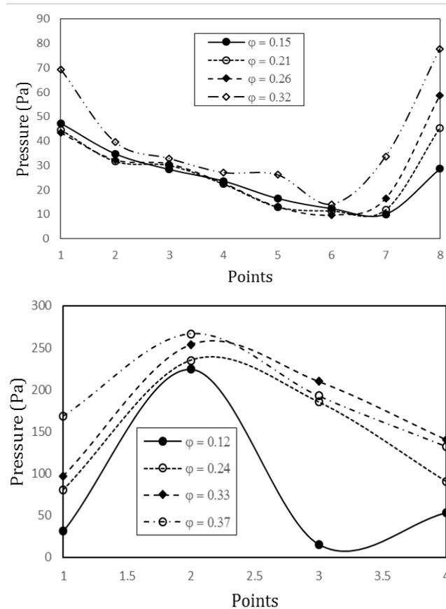
**Fig. 14. Pressure fluctuation amplitude at blade passing frequency on the mid plane of the volute of (a) single outlet and (b) double outlet squirrel cage fan.**
