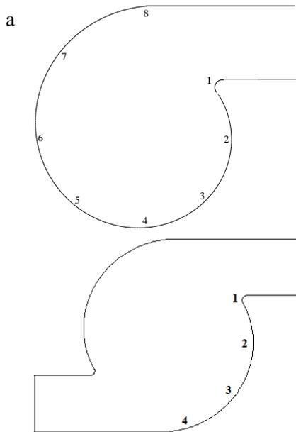
**Fig. 8.** Point of measurement of pressure fluctuations on the mid plane of the (a) single outlet and (b) double outlet squirrel cage fan
