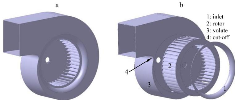
Fig. 1. A view of squirrel cage fan; (a) a complete setup, (b) a detailed view.
