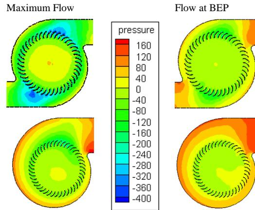
**Fig. 13. Relative static pressure in middle plane of fans at maximum flow rate (left) and flow of BEP (right).**
