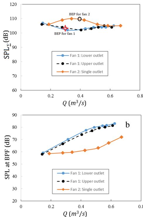
**Fig. 12. Comparison of (a)  $SPL_{\Sigma}$  and (b) blade passing frequency noise of fan 1 and 2.**
