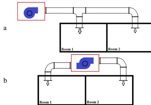
Fig. 3. Applications of (a) double outlet and (b) single outlet squirrel cage fans, in a ventilating system.
