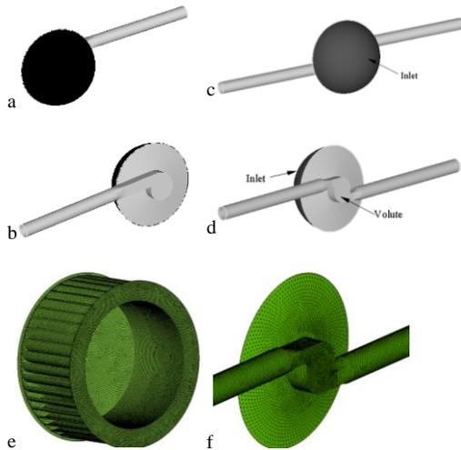
**Fig. 4. Computational domain in numerical simulation of the fans; a: single outlet fan, front view b: single outlet fan, back view; c: double outlet fan, front view d: double outlet fan, back view e: mesh on the rotor f: mesh on the volute and outlets.**
