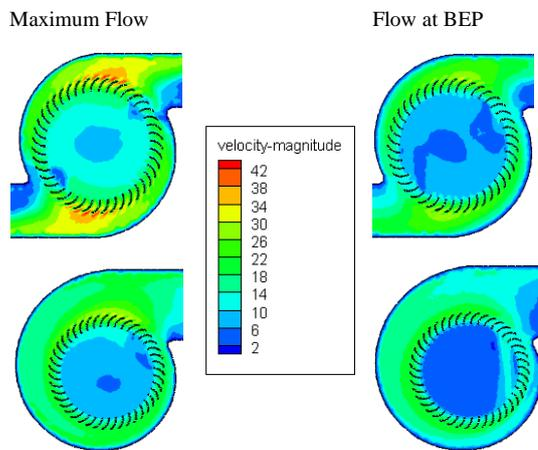
**Fig. 10. Fluid flow (velocity magnitude) in middle plane of fans at maximum flow rate (left) and flow at BEP (right).**
