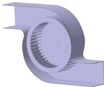
Fig. 2. A schematic view of double outlet squirrel cage fan volute.
