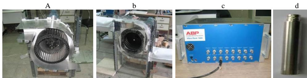
**Fig. 7. Test set and measurement devices, (a) double outlet fan after installation, (b) double outlet fan connected to the ducts, (c) data acquisition front, (d) microphone.**
