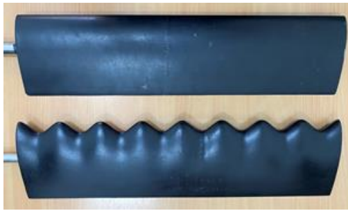
Fig. 7. Baseline and A07W50 Modified Airfoils.
