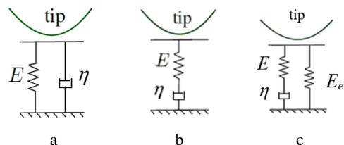
**Fig. 1. Viscoelastic models base on the spring and damper connection a) Kelvin b) Maxwell c) SLS (Iversen, 2015).**
