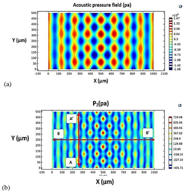
**Fig. 4. First and second order acoustic pressure (a) First order acoustic pressure contour ( $P_1$ ). (b) Second order acoustic pressure ( $P_2$ ).**
