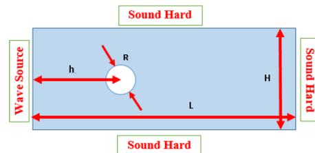
**Fig. 6. Boundary condition and dimensions of the rigid cylinder study.**
