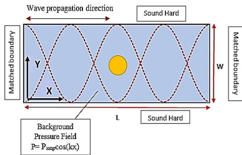
Fig. 2. Geometry and boundary condition of the computational domain.
