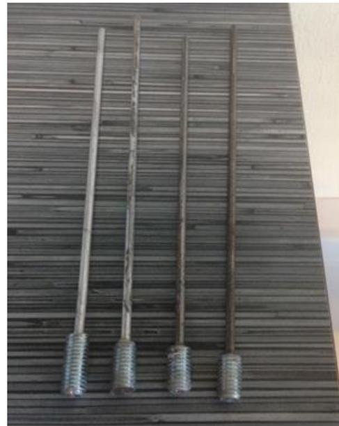
Fig. 6. Aluminium and carbon steel cylinders with  $AR = 50$  and  $54$ .
