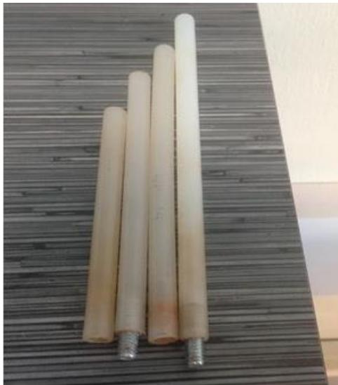
**Fig. 7. Four EVA cylinders with AR = 10, 12, 14 and 16.**
