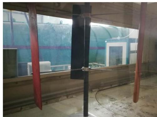
**Fig. 4.** Wind turbine B test model.
